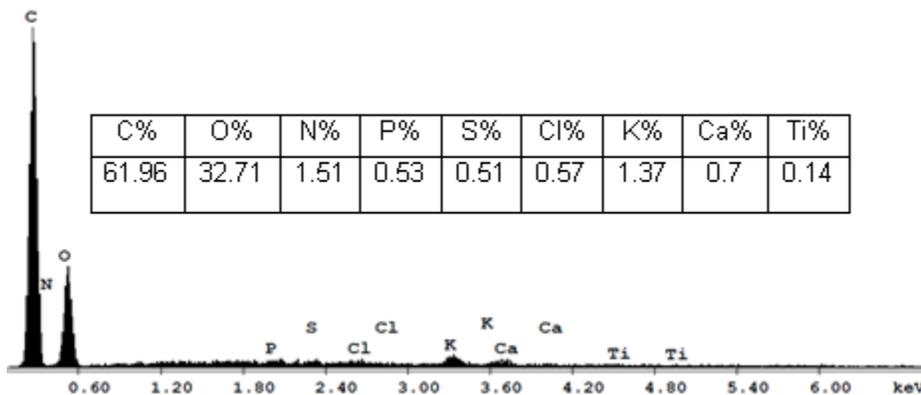
Fig. 3. EDX analysis of treated wood with Paraloid72/TiO<sub>2</sub> nanocomposite at 5%
