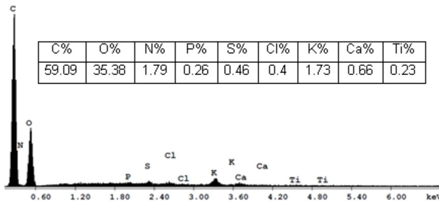
Fig. 4. EDX analysis of treated wood with Paraloid B-72/TiO<sub>2</sub> nanocomposite at 10%
