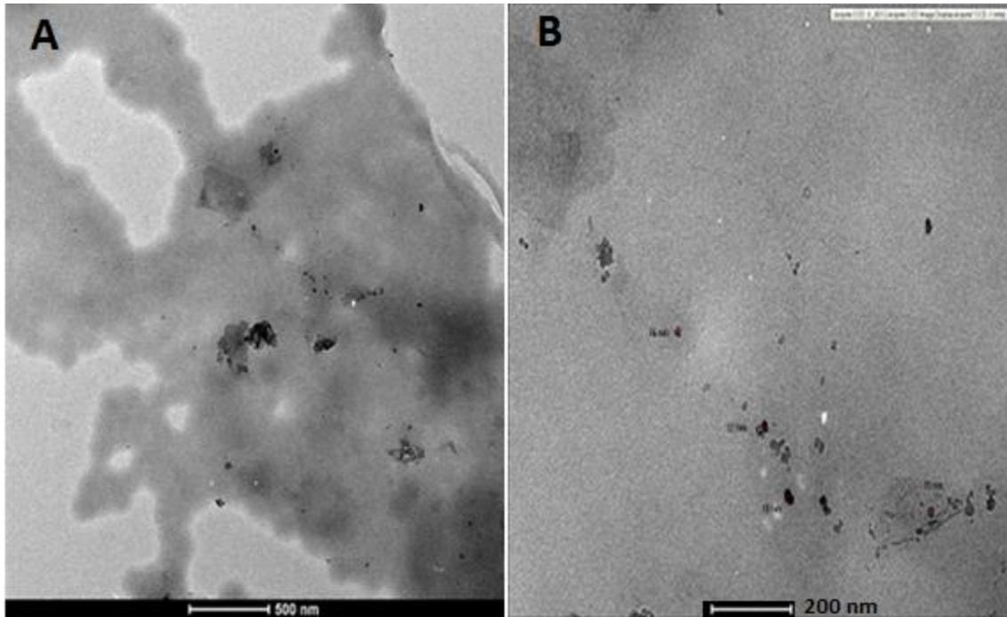
**Fig. 1.** TEM images of nanocomposite for Paraloid B-72 (5%) in presence of 3% TiO<sub>2</sub>; A) Photo at 500 nm of magnification and B) at 200 nm of magnification
