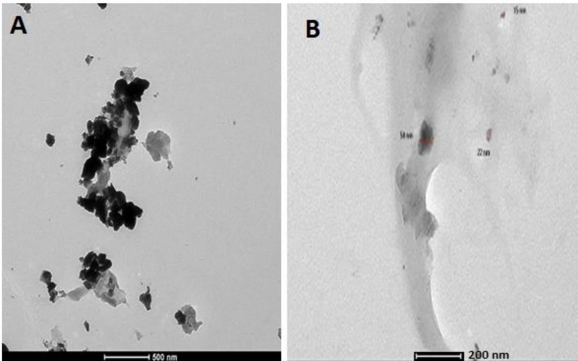
**Fig. 2.** TEM images of nanocomposite for Paraloid B-72 (10%) in presence of 3% TiO<sub>2</sub>; A) Photo at 500 nm of magnification and B) at 200 nm of magnification
