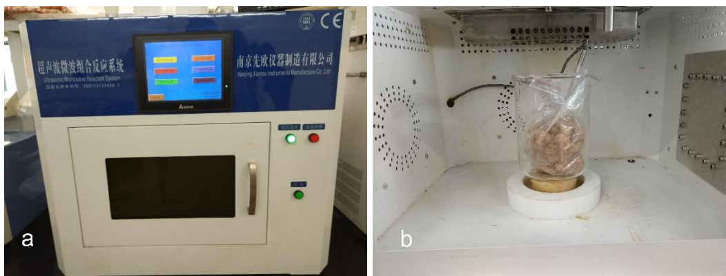
Fig. 1. Microwave apparatus for ClO 2 bleaching: (a) the microwave reaction system, (b) the state of pulp in microwave system.
