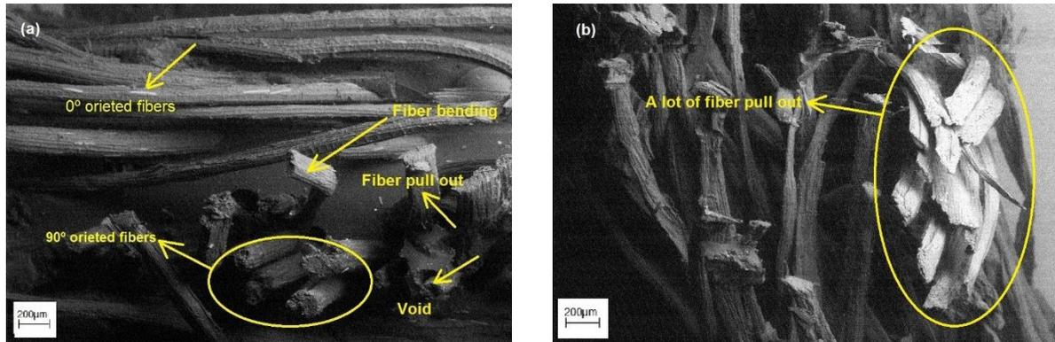
**Fig. 5.** SEM studies on the effect of  $90^\circ / 0^\circ / 0^\circ / 90^\circ$  (a), and  $0^\circ / 90^\circ / 45^\circ / 45^\circ / 90^\circ / 0^\circ$  (b) fiber orientation on the impact strength of sisal fiber composites
