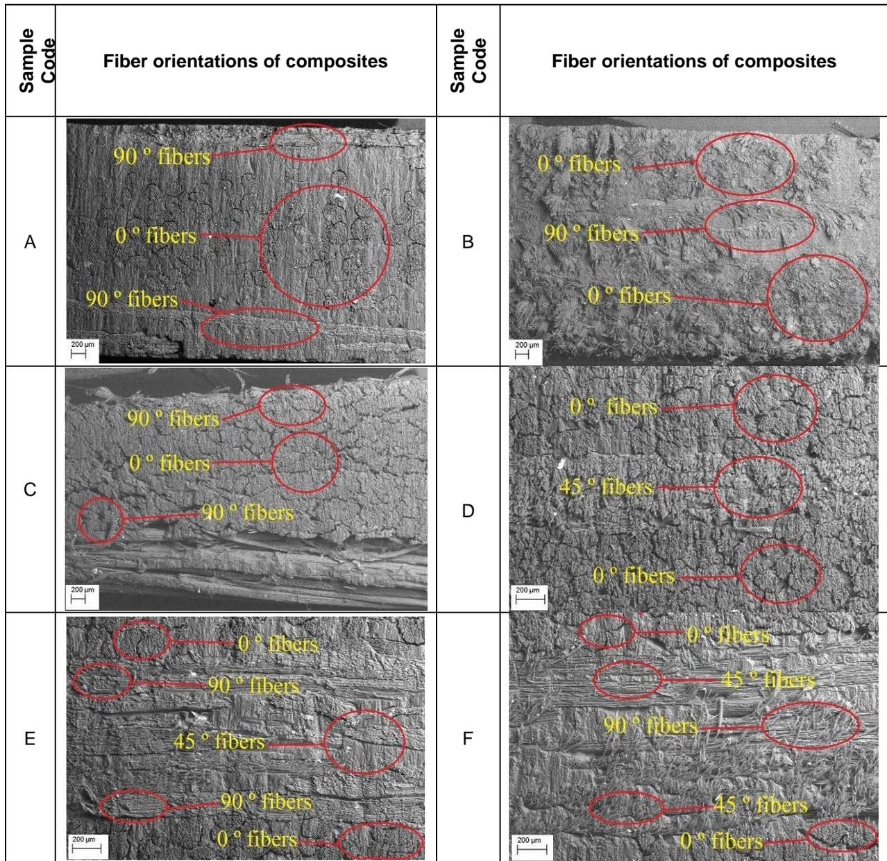
**Fig. 3.** SEM Images of interlaminar fiber orientations
