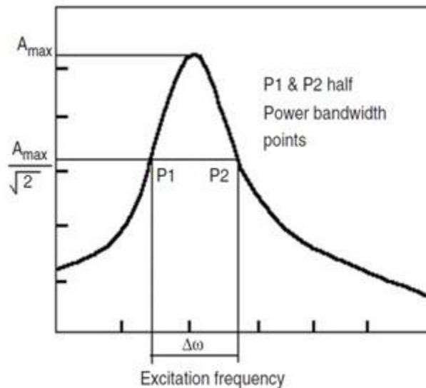
**Fig. 7.** Half-power band method (Chandradass *et al.* 2008)
