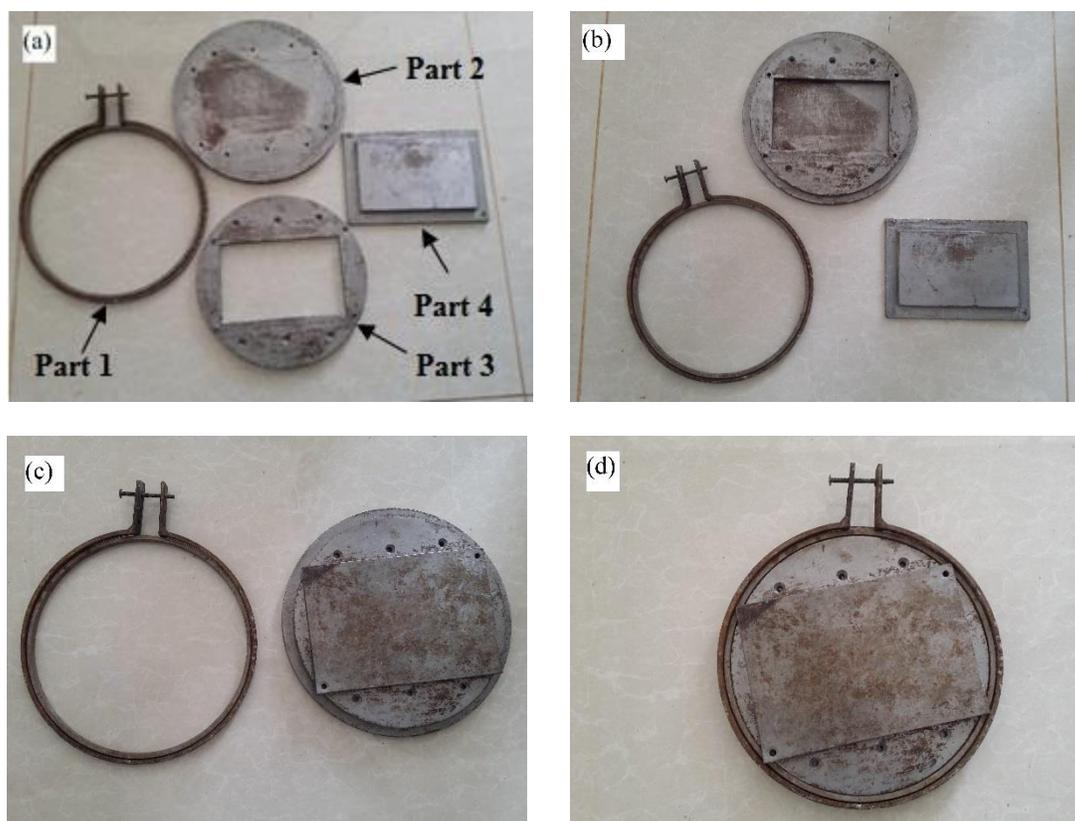
**Fig. 1 (a-d).** Photographic view of different parts of the mold and its various positions in the fiber reorientation process
