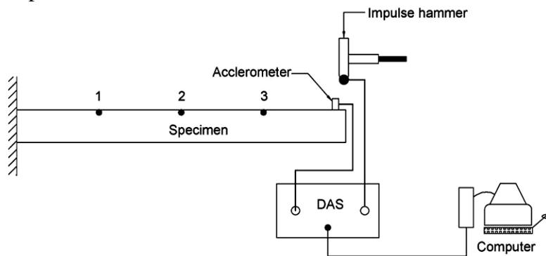
**Fig. 2.** Schematic diagram of free vibration experimental setup
