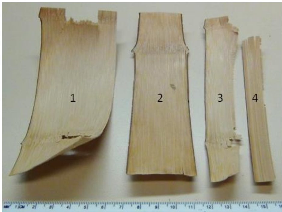
Fig. 3. Examples of real strands (1) strand from close to point r from slicing a half round, (2) strand from close to point R from slicing a full round, (3) full wall strand between points c and r , and (4) full wall strand close to Y -axis slicing halves or quarters
