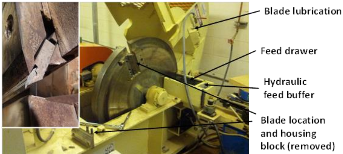
Fig. 1. CAE 6/36 Lab Flaker, disk rotation direction is clock-wise; inset: close up view of disposable twin blade in its housing
