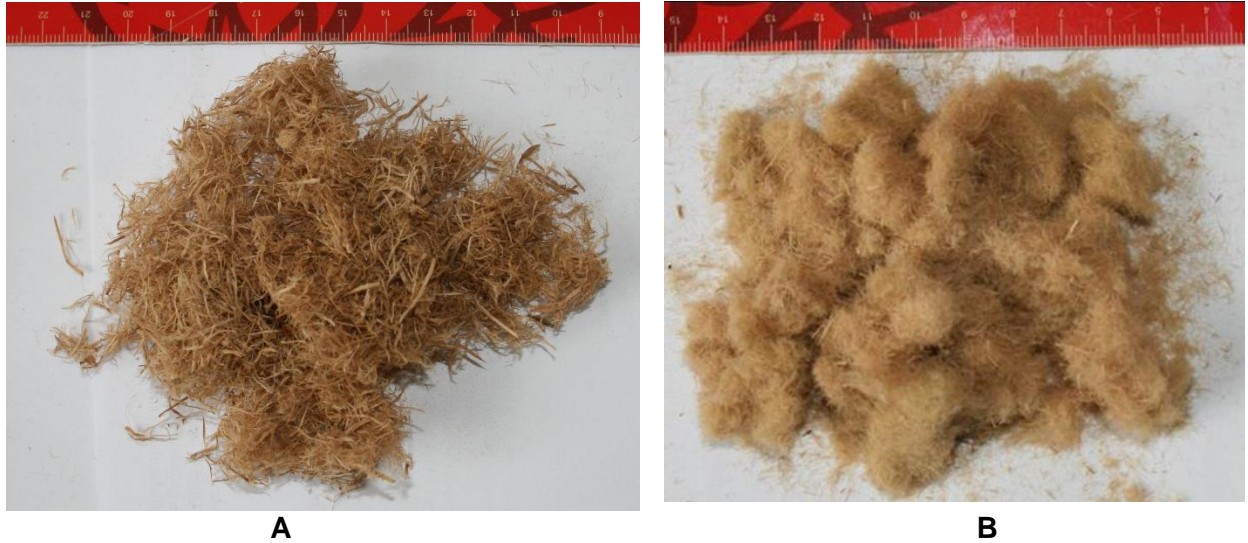
Fig. 1. A: Coarse beech wood fibers used in the core layer of MDF (1.2 mm defibrator discs distance). B: Fine pine wood fibers used in the face layers of MDF (0.4 mm defibrator discs distance)
