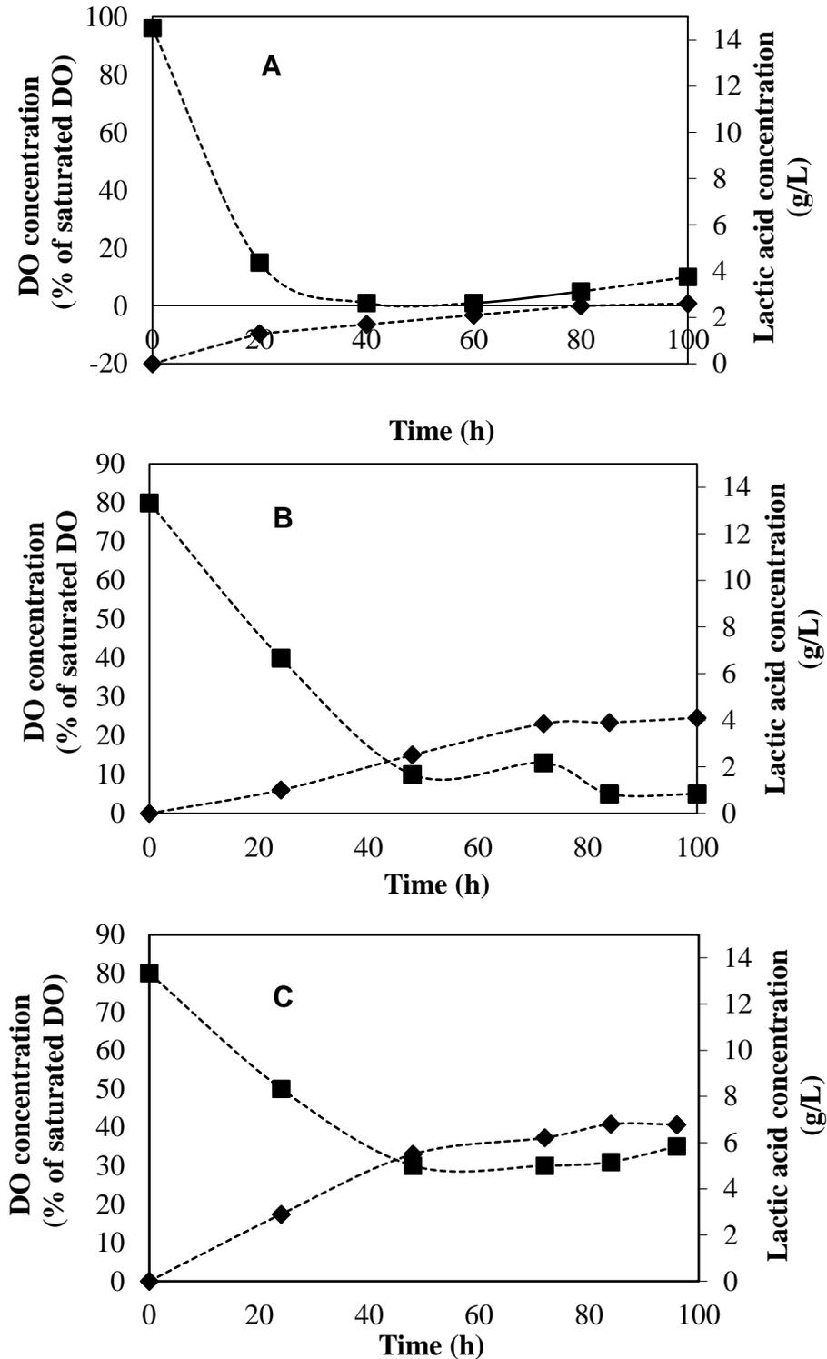
**Fig. 4.** Lactic acid fermentation profiles in 150-L scale at different  $V_s$  values: (A)  $V_s = 0.2$  cm/s,  $k_L a = 0.011$ , (B)  $V_s = 0.5$  cm/s,  $k_L a = 0.039$  and (C)  $V_s = 0.9$  cm/s,  $k_L a = 0.061$ . (♦) Lactic acid concentration, (■) DO concentration
