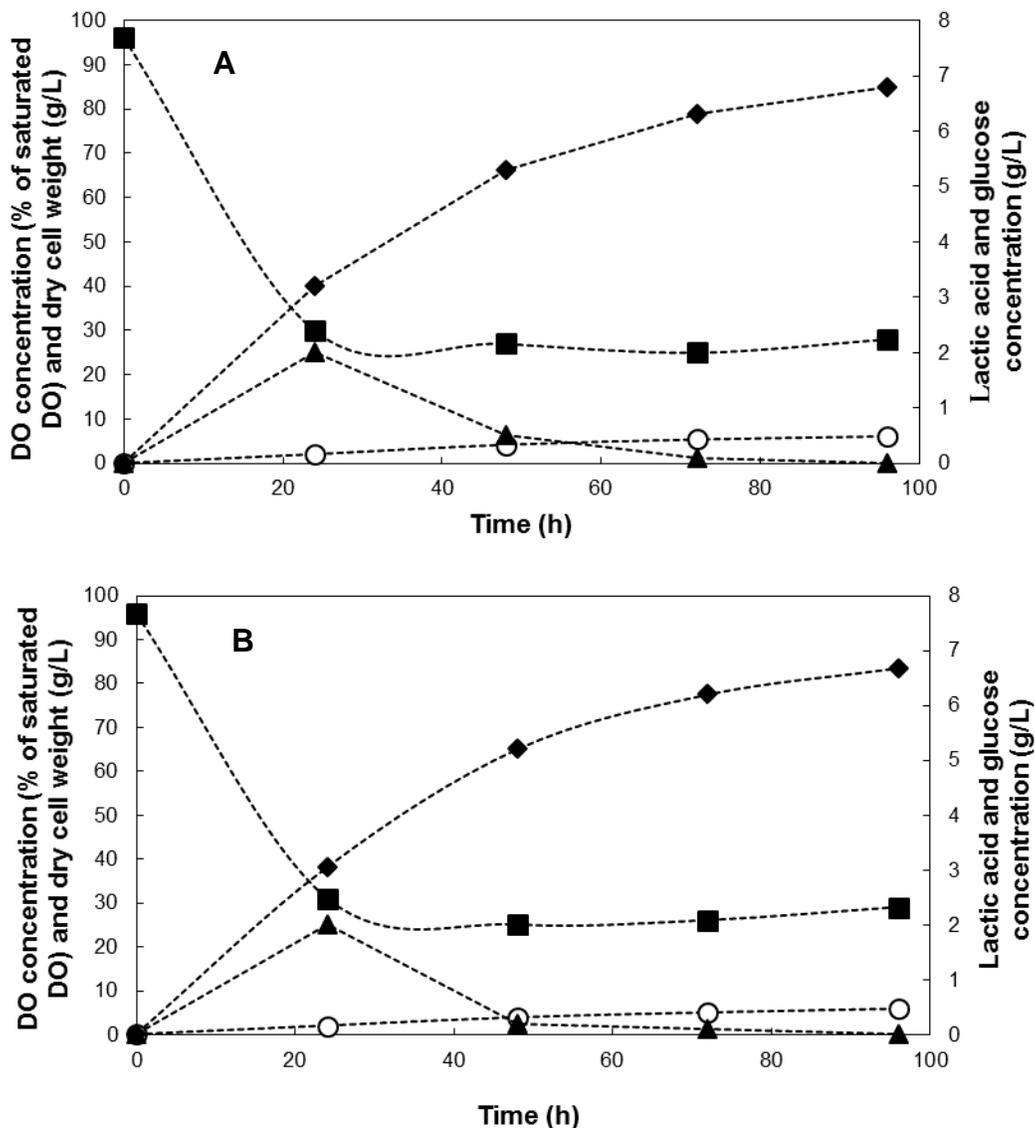
**Fig. 5.** Time-course profiles of cell growth, sugar consumption, DO concentration, and lactic acid production at the same  $k_{La}$  value, (A) in the 16-L fermenter and (B) in the 150-L pilot-scale fermenter; (◆) Lactic acid, (■) DO, (▲) Glucose, (○) Dry cell weight
