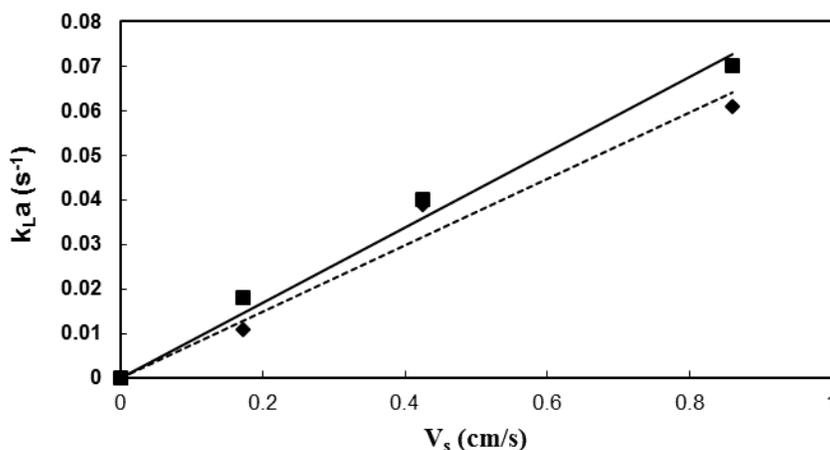
**Fig. 3.** A correlation between  $k_{LA}$  and  $V_s$  in the 16-L and 150-L airlift bioreactors; (♦) 16-L bioreactor, (■) 150-L bioreactor
