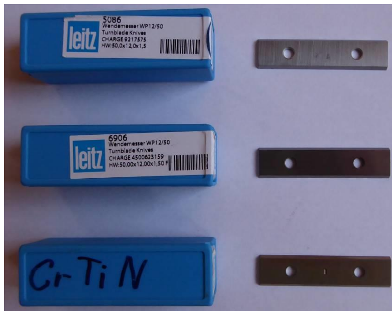
Fig. 2. Blade types for edge milling
