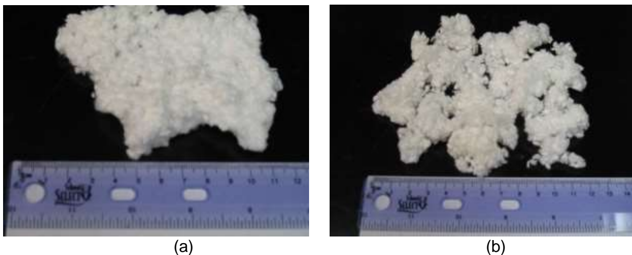
Fig. 2. Photographs of (a) forced-air dried ethanol pulps and (b) forced-air dried and milled ethanol pulps.
