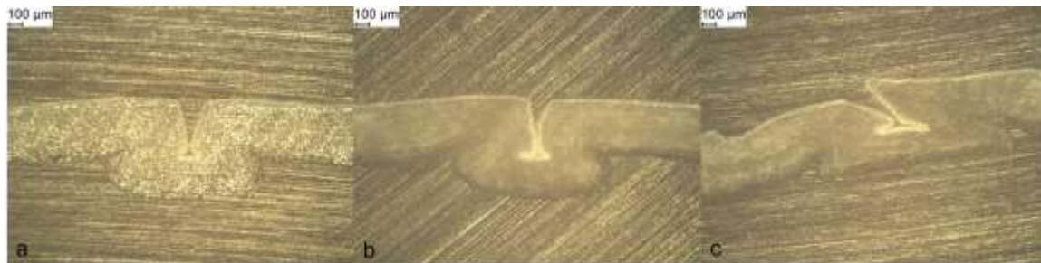
Fig. 6. Cross-section of single formed creases before sealing in trays manufactured with different blank holding forces: a) 1000 N, b) 750 N, and c) 500 N
