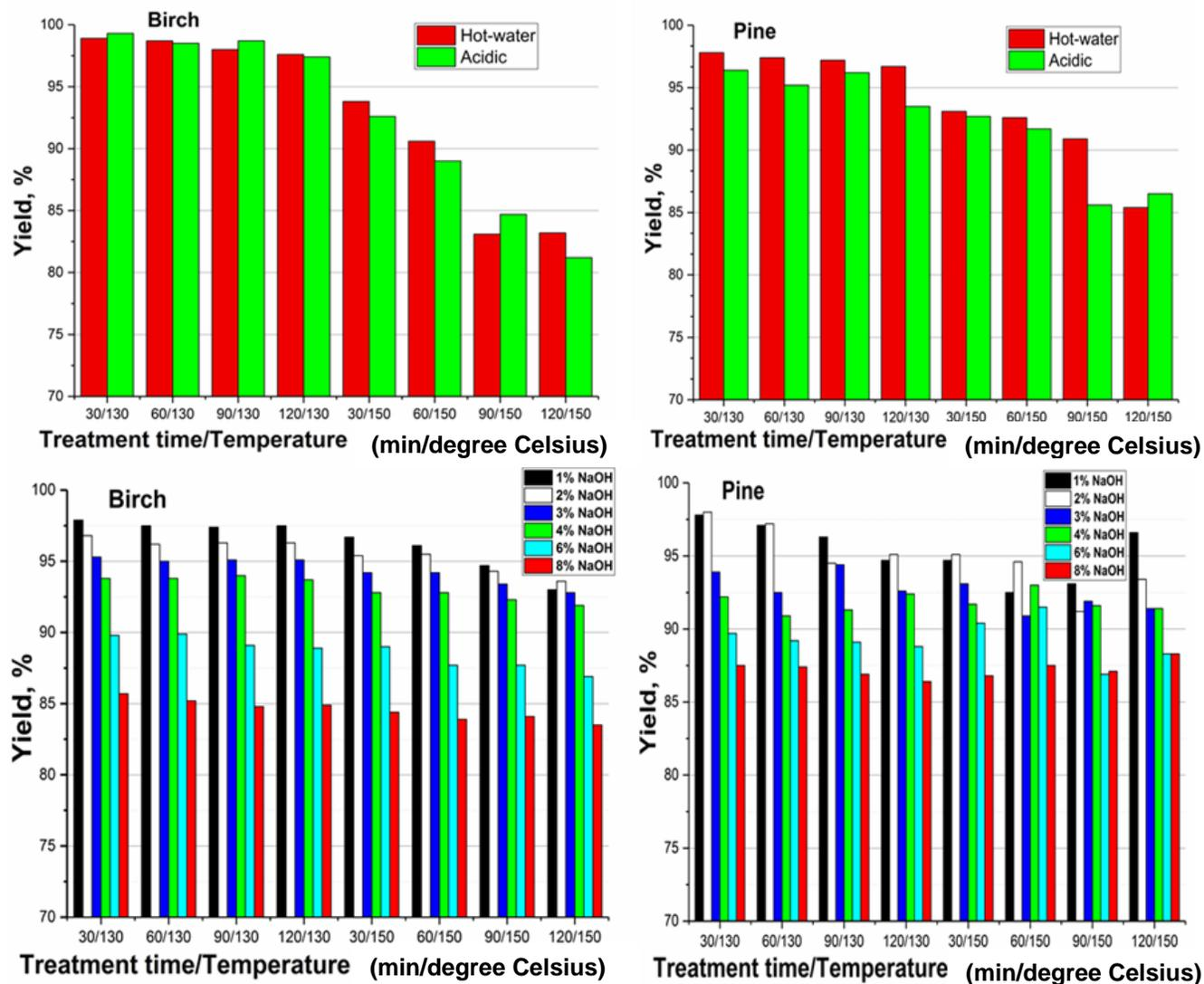
Fig. 1. Yield (% of original dry wood) data on autohydrolysis (top) and alkaline (bottom) pre-treatments
