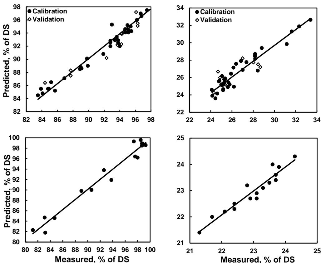
**Fig. 3.** Predicted vs. measured yield (left) and lignin content (right) of the alkaline (upper) and autohydrolysis (lower) pre-treated birch chips
