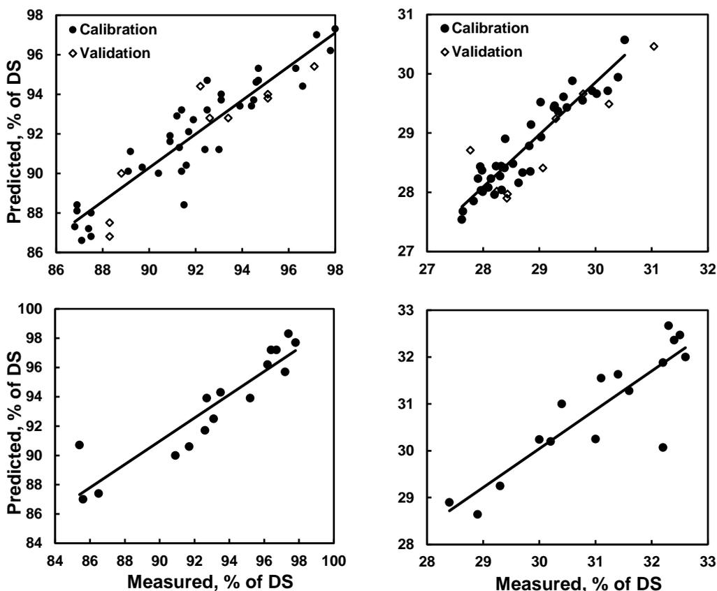
Fig. 4. Predicted vs. measured yield (left) and lignin content (right) of the alkaline (upper) and autohydrolysis (lower) pre-treated pine chips
