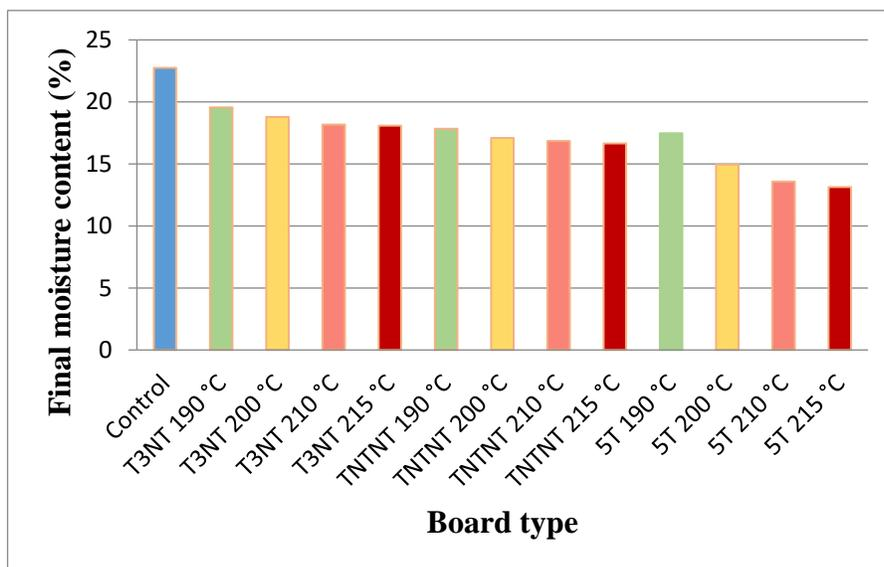
Fig. 4. Influence of board construction and treatment temperature on final moisture content
