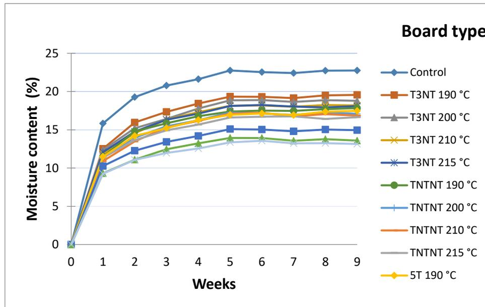
**Fig. 2.** Moisture content change curves of board samples above water
