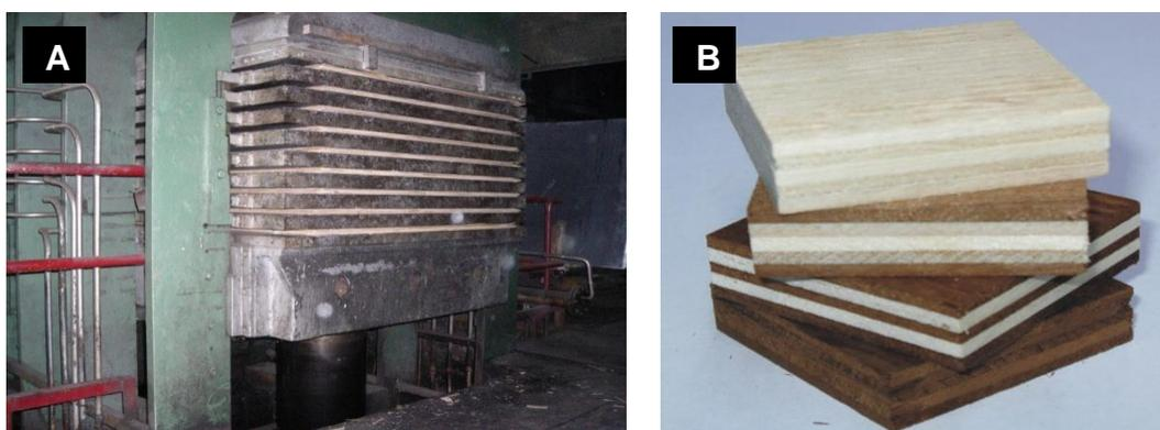
**Fig. 1.** Board pressing (A) and types of pressed boards (B)
