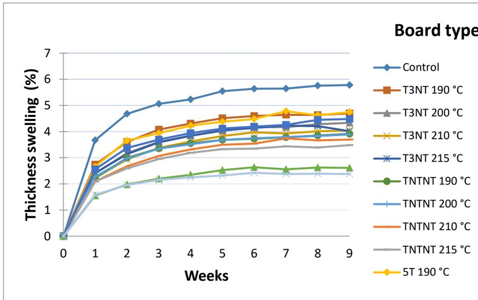
Fig. 3. Curves of thickness swelling of boards samples above water
