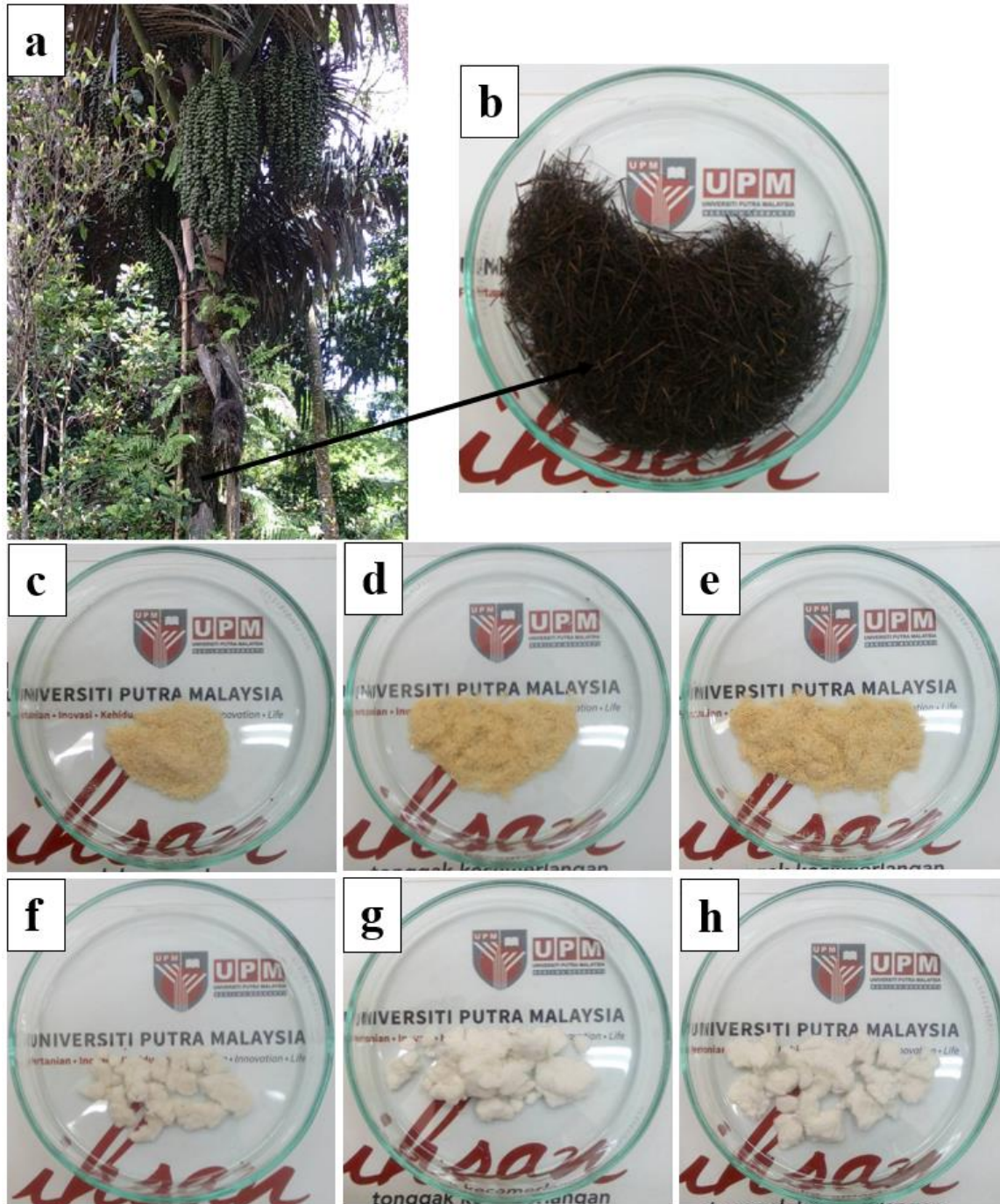
Fig. 1. Photographs of the (a) sugar palm tree; (b) raw SPF; bleached fibre: (c) SPBF05, (d) SPBF06, and (e) SPBF07; and alkali-treated fibre: (f) SPC05, (g) SPC06, and (h) SPC07
