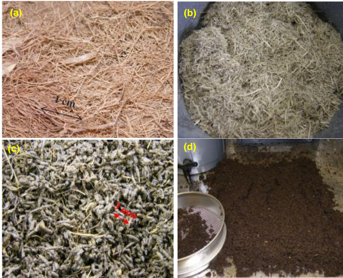
Fig. 7. Physical changes of EFB from raw material to vermicompost; (a) raw EFB (control), (b) treated EFB with P. sajor-caju , (c) vermicasts, and (d) EFB vermicompost after 30 weeks of composting
