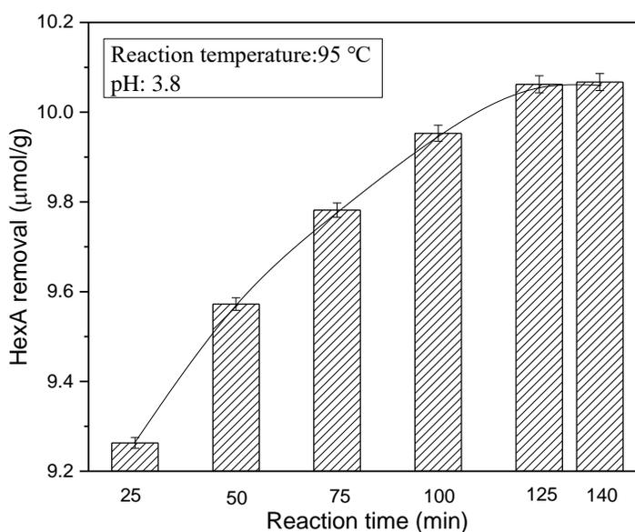
**Fig. 2.** Impact of reaction time on HexA removal
