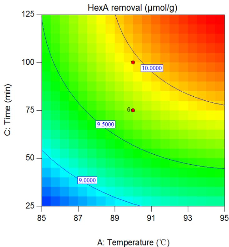
**Fig. 5.** Three-dimensional response surface plot and isopleth diagram for HexA removal based on reaction temperature and reaction time
