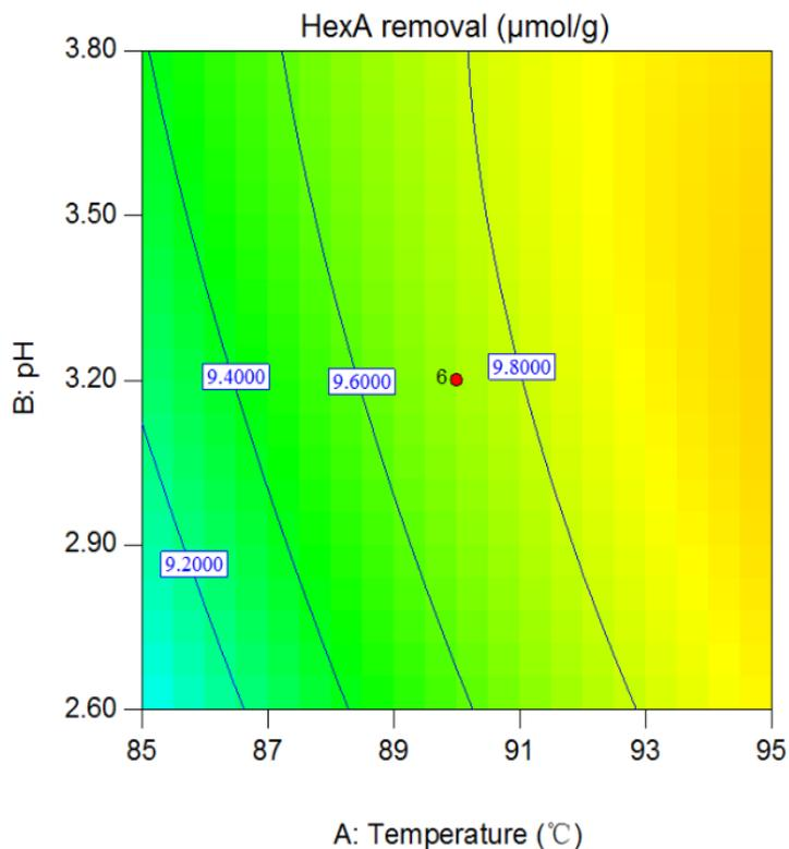
**Fig. 4.** Three-dimensional response surface plot and isopleth diagram for HexA removal based on reaction temperature and pH
