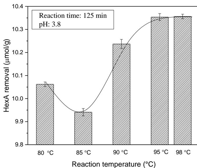
**Fig. 1.** Impact of reaction temperature on HexA removal
