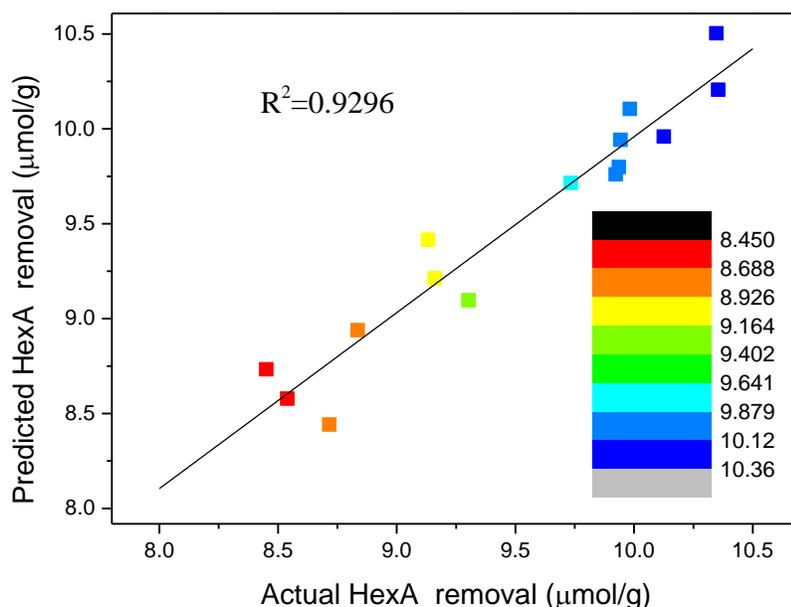
**Fig. 8.** Plotted relation between the predicted and actual values of HexA removal based on response surface model
