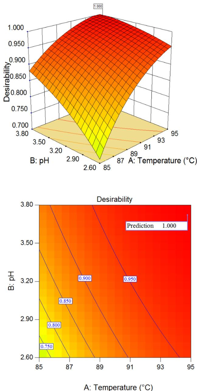
**Fig. 7.** Three-dimensional response surface plot and isopleth diagram for desirability of HexA removal based on reaction temperature and pH
