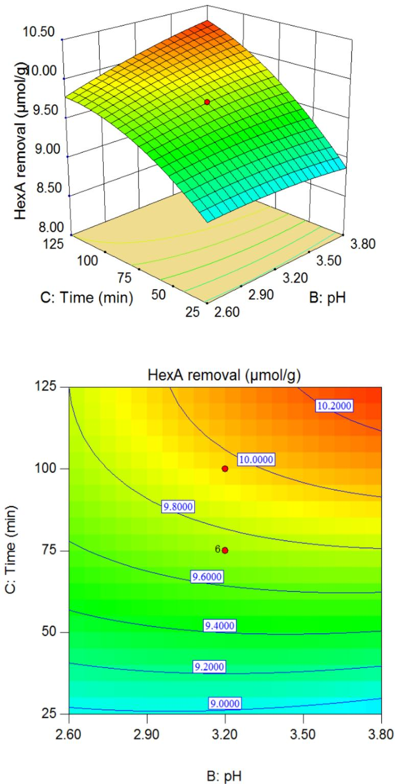
**Fig. 6.** Three-dimensional response surface plot and isopleth diagram for HexA removal based on pH and reaction time
