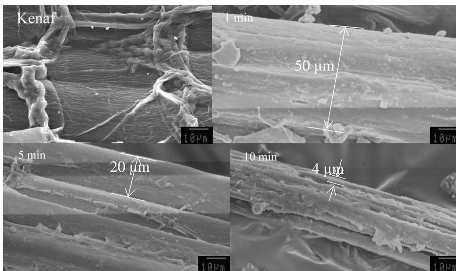
**Fig. 3.** SEM images of kenaf (fiber) after different residence time steam explosion treatment
