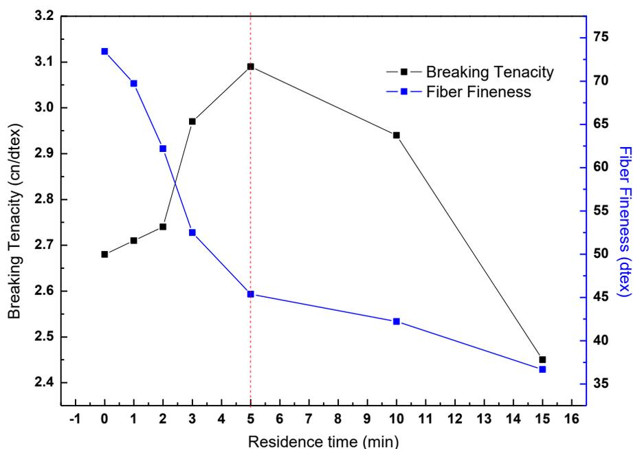
**Fig. 6.** Breaking tenacity and fiber diameter of kenaf fiber after different residence time steam explosion treatments
