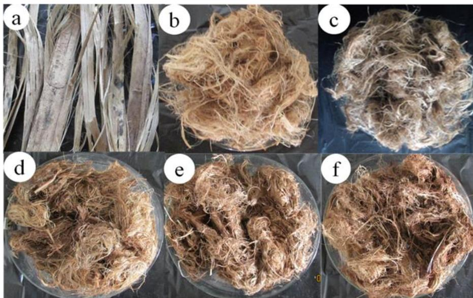
**Fig. 2.** Photograph of kenaf (fiber) after different residence time steam explosion treatment (a) raw kenaf, (b) 1 min, (c) 3 min, (d) 5 min, (e) 10 min, and (f) 15 min
