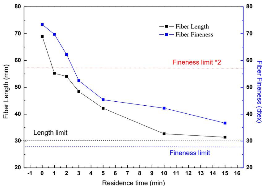
**Fig. 5.** Fiber length and diameter of kenaf fiber after different residence time steam explosion treatments
