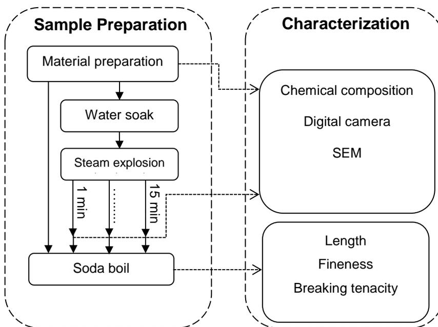
Fig. 1. Schematic diagram for the degumming and characterization process
