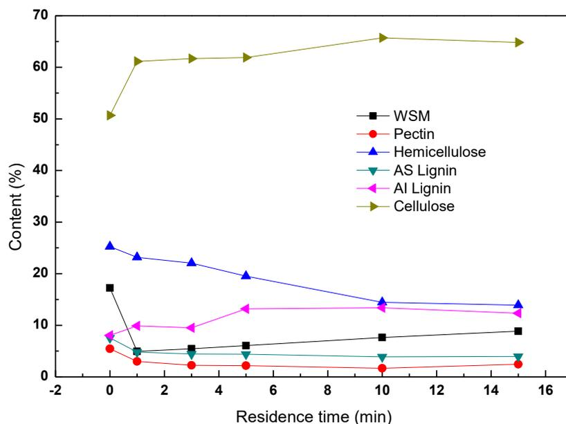
**Fig. 4.** Chemical composition of kenaf after different residence time steam explosion treatments; Note: WSM represents water soluble matter, AS represents acid soluble, Al represents acid insoluble
