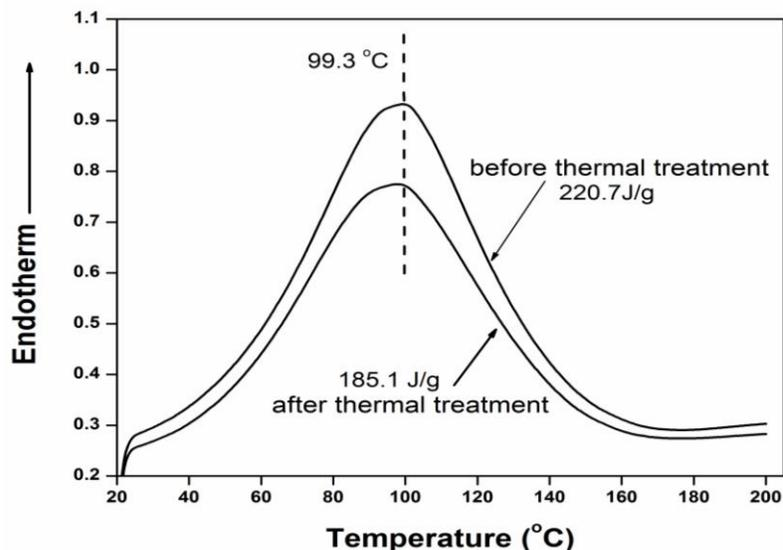
Fig. 4. The DSC curves of the carbon fiber paper before and after thermal treatment
