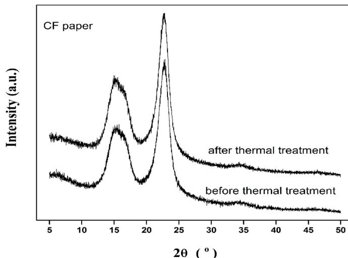
**Fig. 3.** XRD patterns of the carbon fiber paper before and after thermal treatment
