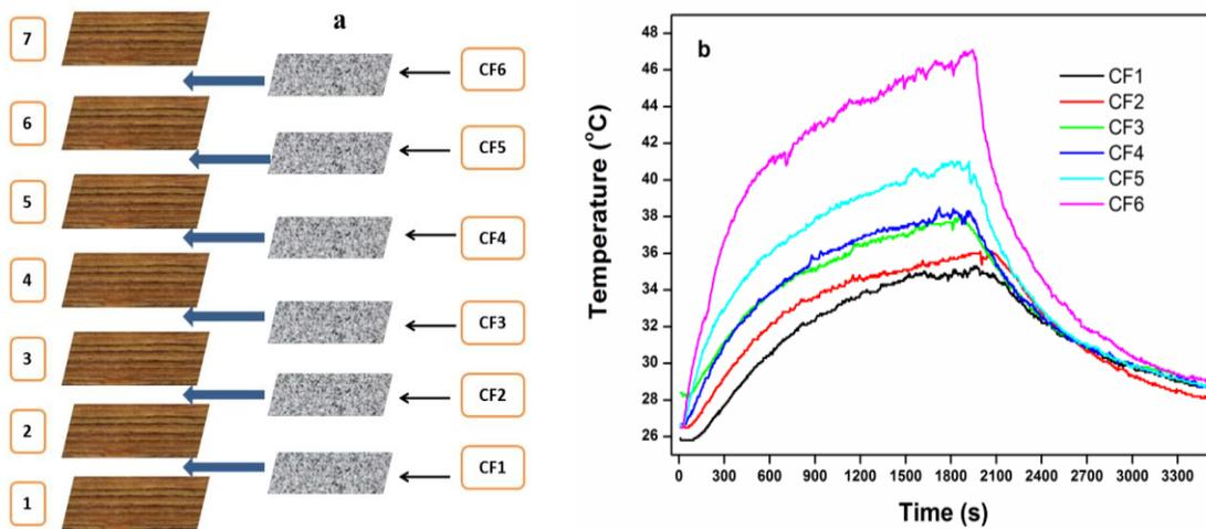
Fig. 6. (a) A sketch of CF paper position in electric heating wood floors; (b) the heating curves of the electric heating wood floors with different CF paper positions
