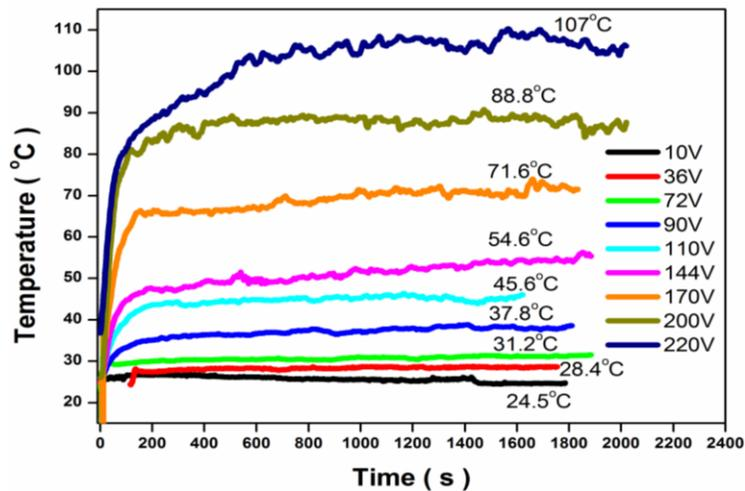
Fig. 5. The electric heating curves of the carbon fiber paper with different input voltages
