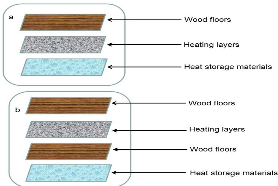
**Fig. 1.** Heating floors with the heating layers (a) below and (b) in the floors
