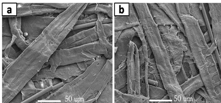
**Fig. 2.** SEM images of carbon fiber paper (a) before and (b) after thermal treatment
