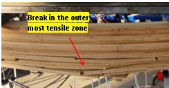
Fig. 6. Typical failure mode of LB beam
