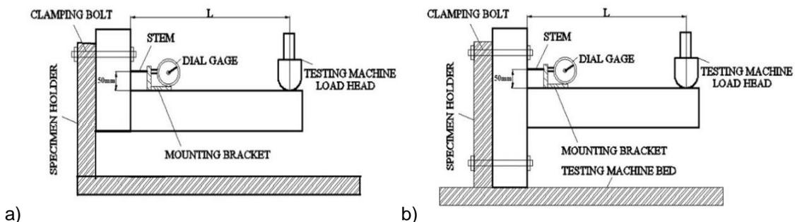
**Fig. 5.** Diagrams showing the bending loading forms and attachments of (a) L- and (b) T-shaped joint specimens to the test rig
