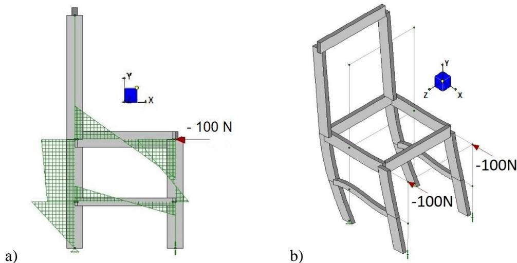
**Fig. 8.** Bending moment diagram (a) and exaggerated deflected shape (b) of the chair frames
