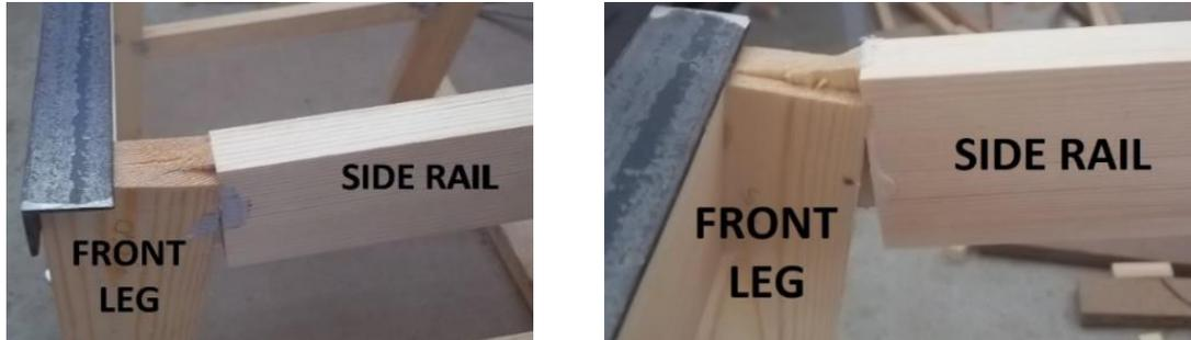
**Fig. 7.** Typical failure modes of the chair frames including the first failed joint
