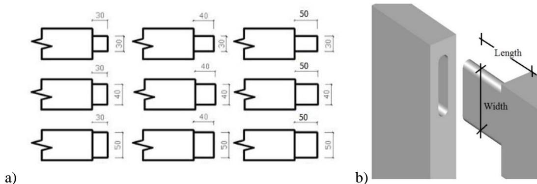
**Fig. 2.** Geometries of the various sizes of mortise and tenon joints (a) and detail of round edge (b) of the mortise and tenon joint; measurements in mm
