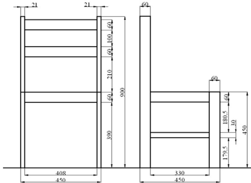
**Fig. 1.** Dimensions of the chair used in the tests (measurements in mm)
