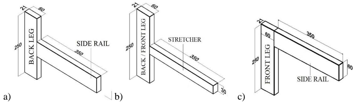
**Fig. 3.** T-type (a, b) and L-type (c) specimens; measurements in *mm*
