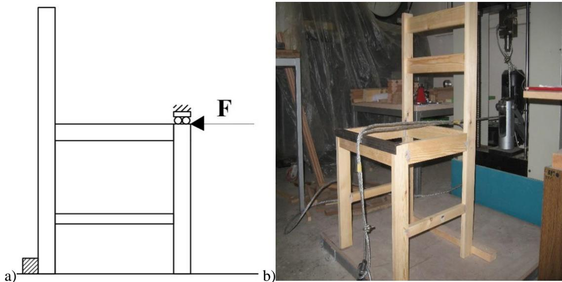
**Fig. 4.** Side view illustration of front to back loading of chair (a), and loading configurations of real chair tests (b)
