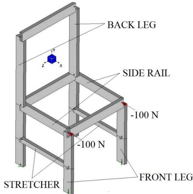
**Fig. 6.** Graphical representation of load application and constraints of DOF on a typical chair frame loaded under front to back direction
