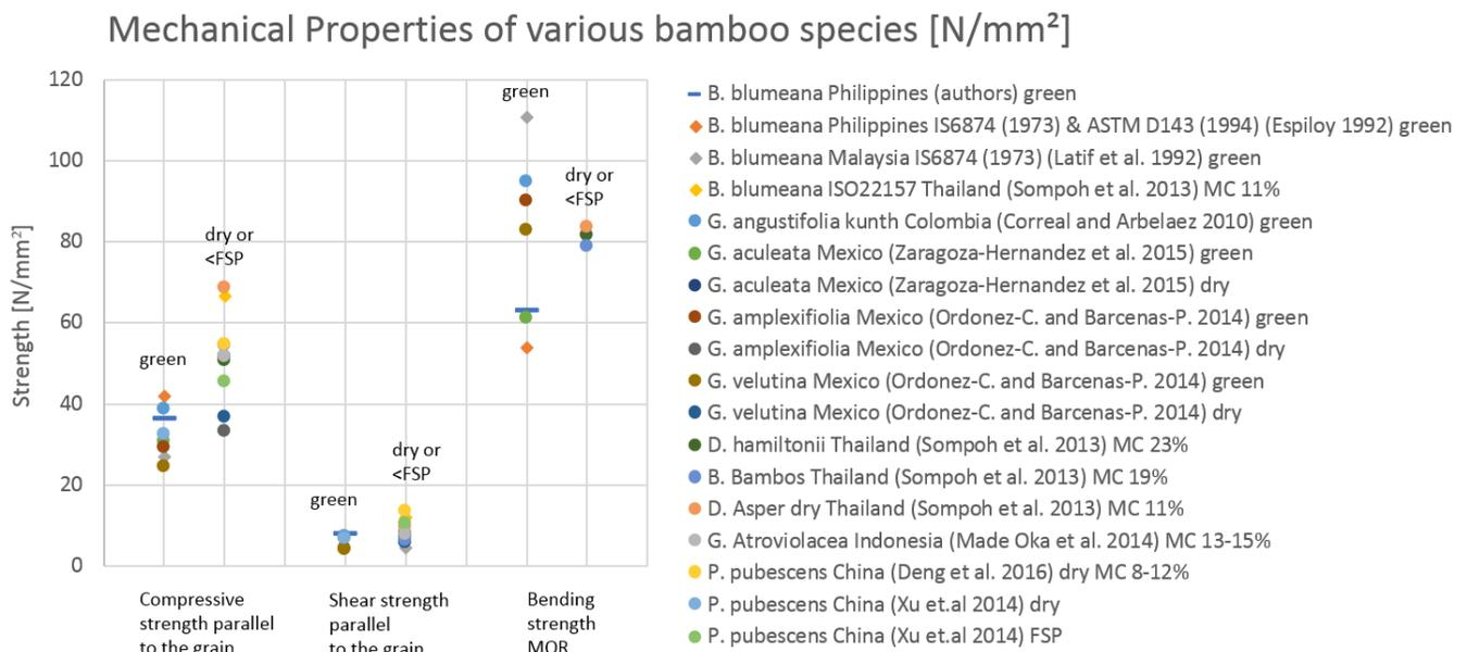
Fig. 2. Mechanical Properties of various bamboo species, including *B. blumeana*, in [N/mm<sup>2</sup>]
