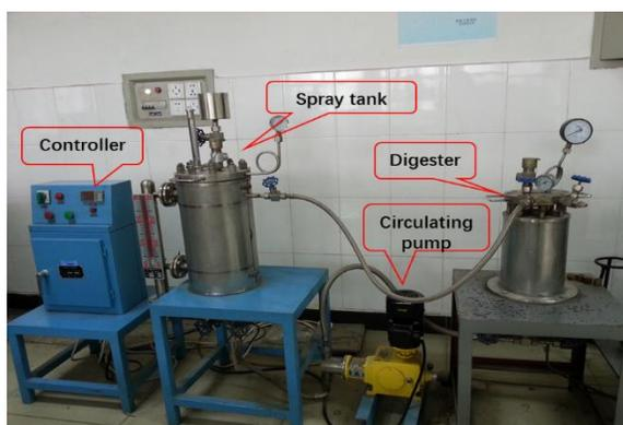
**Fig. 1.** The DDS cooking digester
