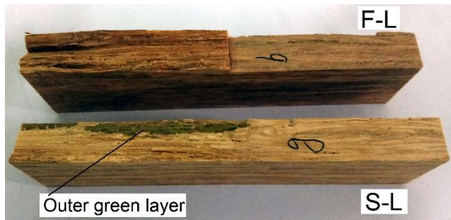
Fig. 7. Comparison of the failure surfaces between two types of specimens
