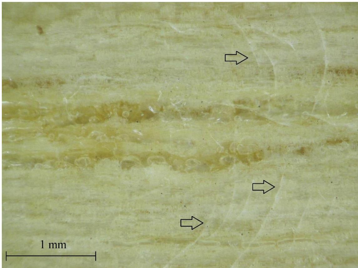
**Fig. 3.** Cracking visible on the surfaces of ash veneer with hydrophilic silicone resin coating after impact resistance testing at the drop height of 400 mm (visible at magnification 35×)
