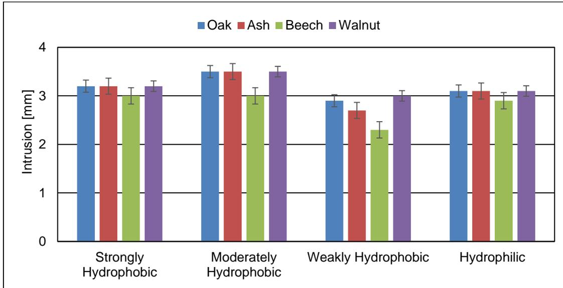
**Fig. 2.** Diameters of intrusions in silicone coatings on various wood species at a drop height of 400 mm
