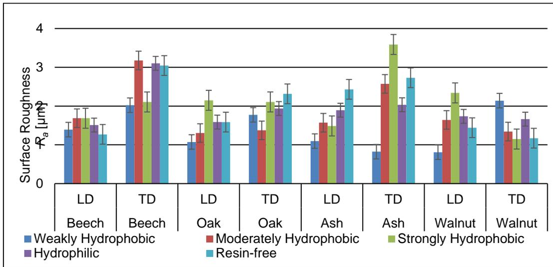
**Fig. 1.** Influence of the interaction between wood species and the type of silicone resin on the roughness (Note: arithmetic mean deviation of the profile  $R_a$ , measured in two directions: longitudinal (LD) with wood fibers and transversal (TD) direction, before and after modification with silicone resins, in traverse length of 0.8 mm)
