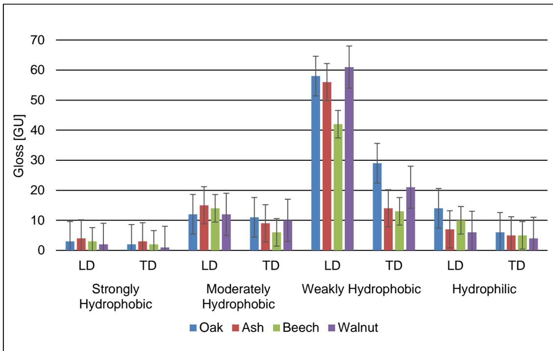
**Fig. 5.** The gloss of veneer surface coated with silicone resins; longitudinal (LD) and transversal (TD) directions
