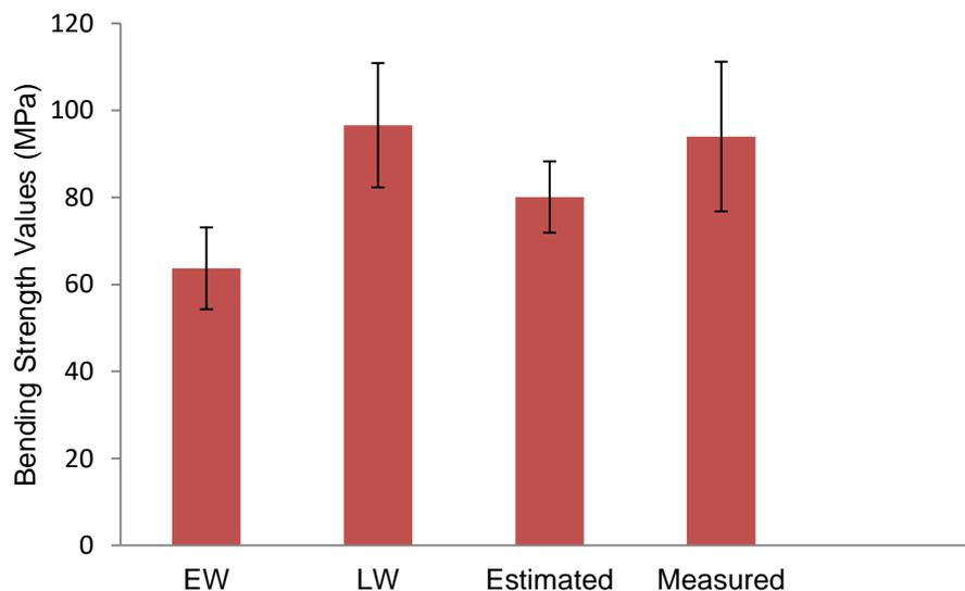
**Fig. 1.** The EW, LW, estimated, and measured bending strength values of oak wood
