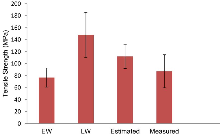
**Fig. 3.** The EW, LW, estimated, and measured tensile strength values of oak wood
