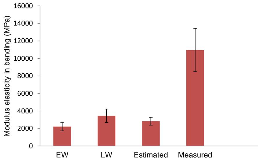
**Fig. 2.** The EW, LW, estimated, and measured MOE values of oak wood
