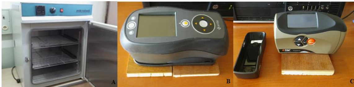
Fig. 1. (A) Mikrotest MST Series Oven, (B) Portable Spectrophotometer X-Rite Ci62 Series, and (C) Glossmeter Poly-gloss GL0030 TQC
