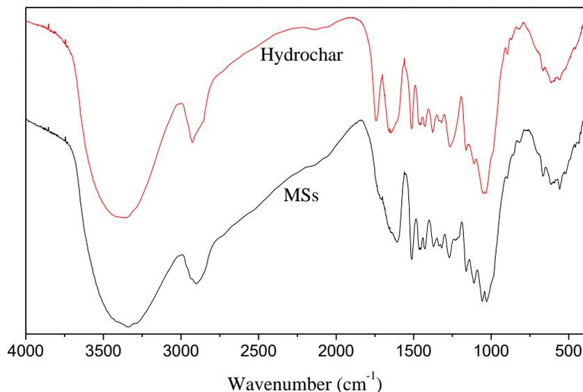
**Fig. 5.** Fourier transform infrared spectra of MSs and their hydrochar at optimum conditions
