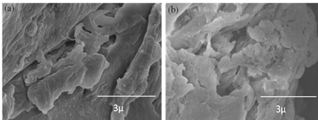
**Fig. 4.** Scanning electron microscopy images of raw MSs (a) and their hydrochar (b) at optimum conditions
