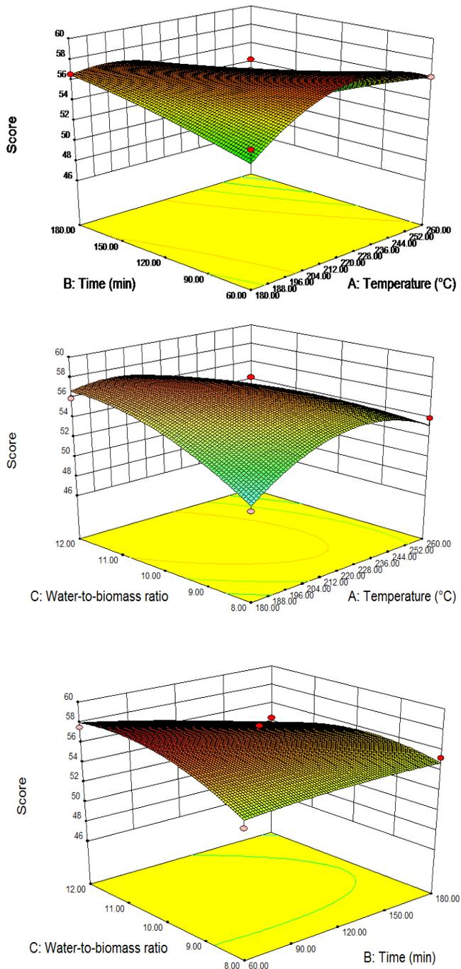
**Fig. 3.** Response surface on the synthetic score. Effect of (a) temperature and time, (b) temperature and water-to-biomass ratio, and (c) time and water-to-biomass ratio
