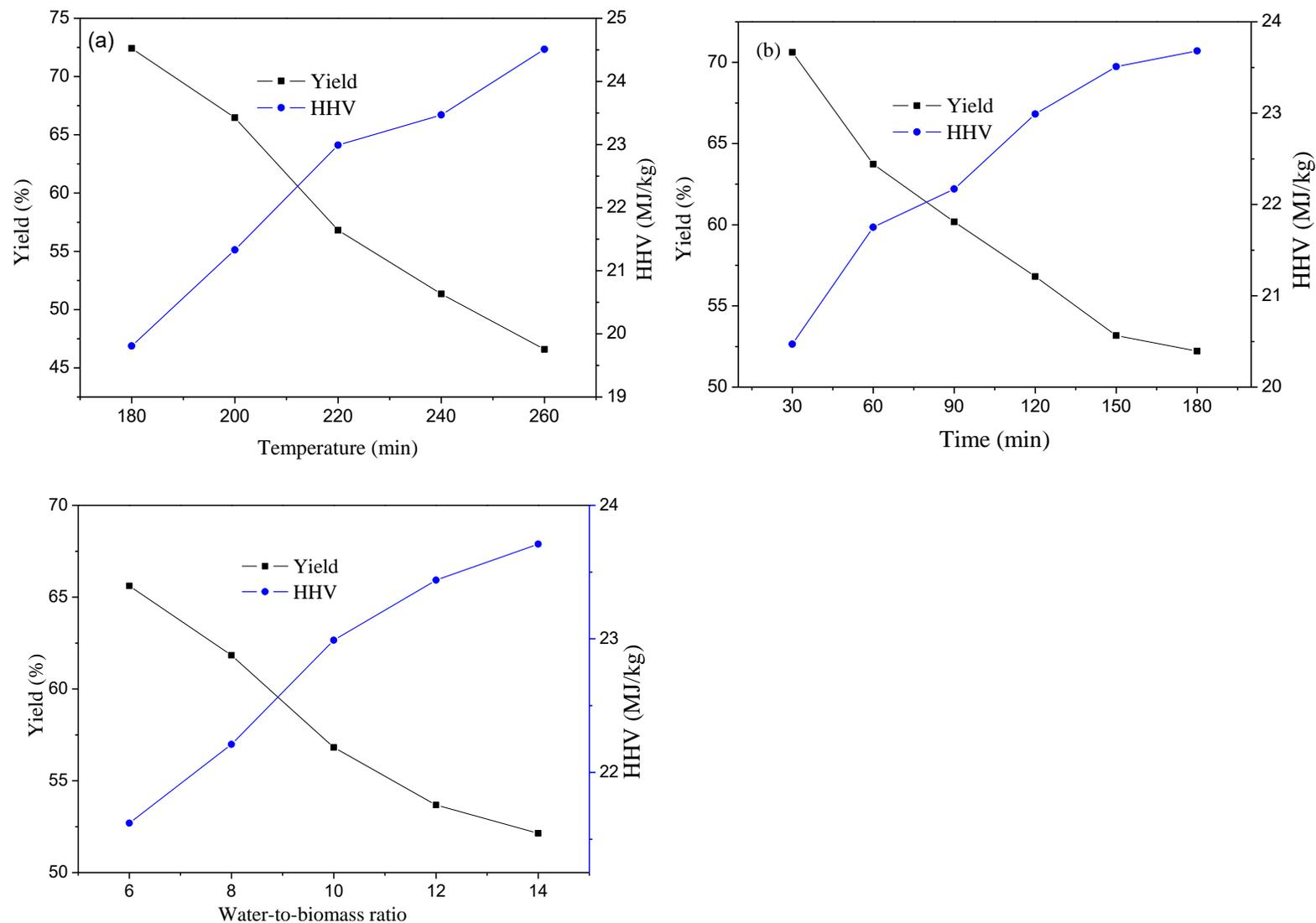
Fig. 1. Effect of (a) reaction temperature, (b) reaction time, and (c) water-to-biomass ratio on the yield and HHV of hydrochar
