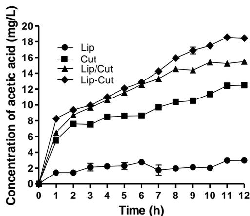
**Fig. 3.** Release of acetic acid from the PVAC after degradation by the Lip, Cut, Lip/Cut mixture, and chimeric Lip-Cut; values shown are the means of the results of the triplicate experiments  $\pm$  the SE
