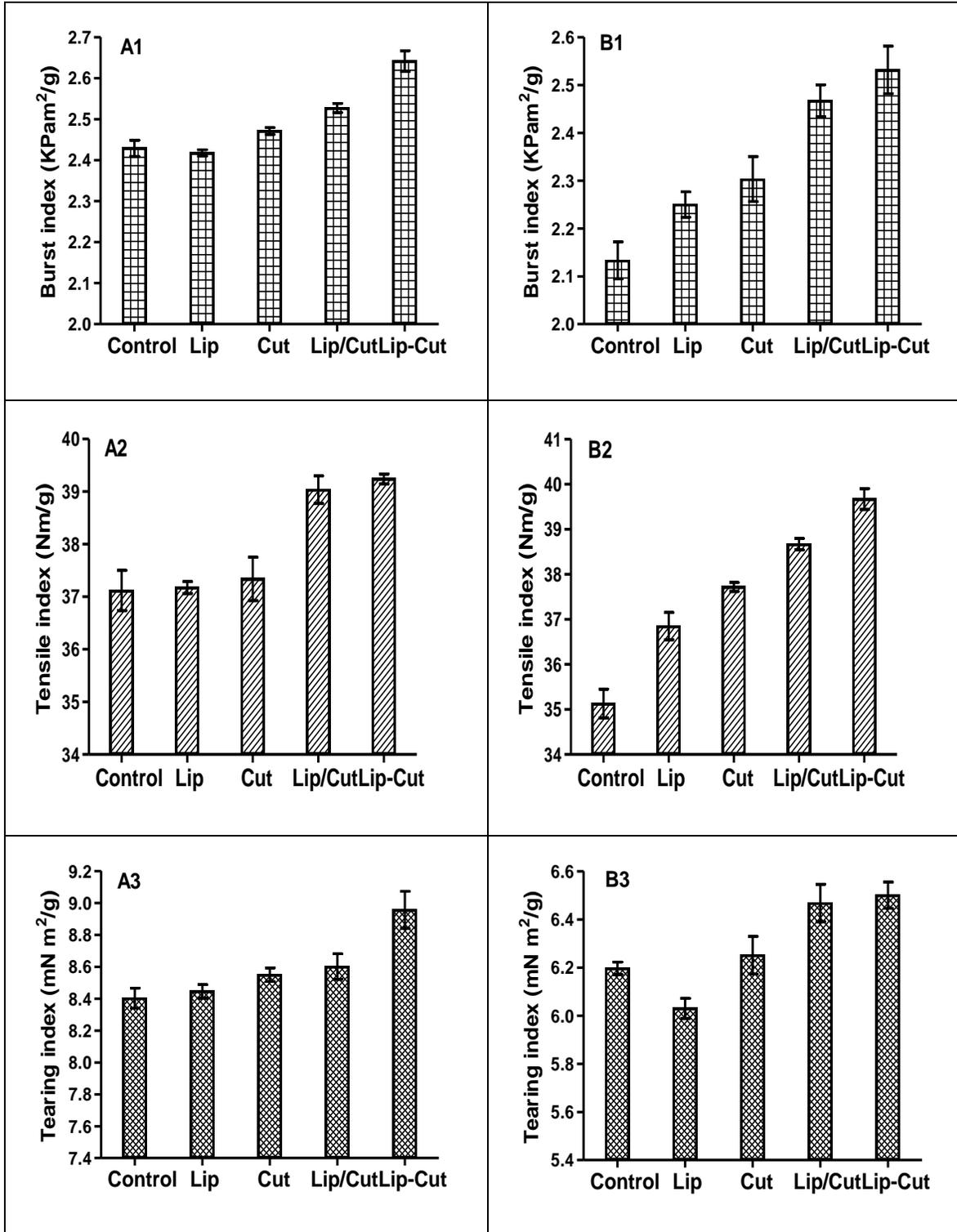
Fig. 5. Strength properties of the deinked laser-printed paper (A) and newspaper (B) after enzyme treatment; A1 and B1: burst index; A2 and B2: tensile index; and A3 and B3: tear index
