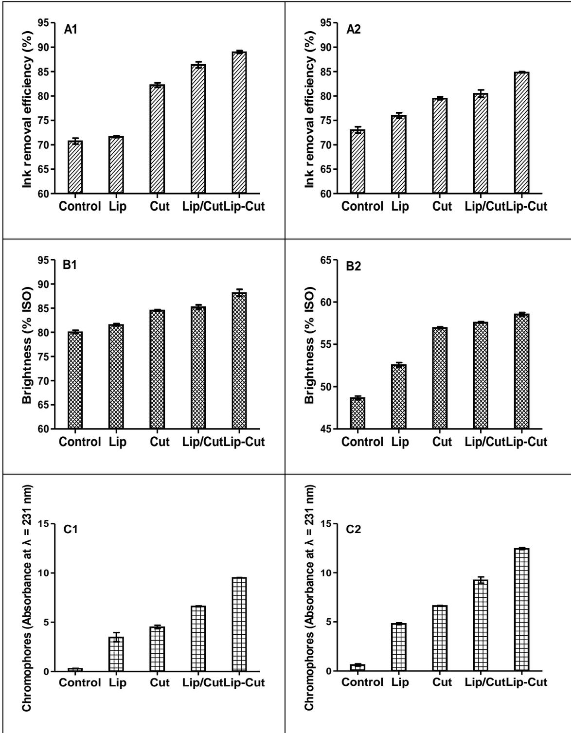
**Fig. 4.** Ink removal efficiencies of the laser-printed paper (A1) and newspaper (A2); brightness of the laser-printed paper (B1) and newspaper (B2); released chromophores in the effluent of the laser-printed paper (C1) and newspaper (C2)
