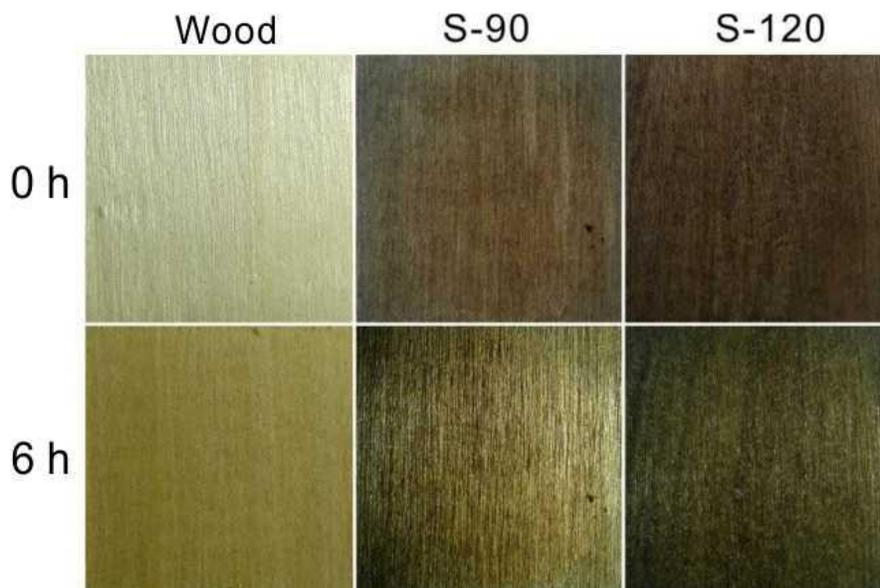
**Fig. 5.** Photographs of untreated wood, S-90, and S-120 before and after 6 h UV irradiation
