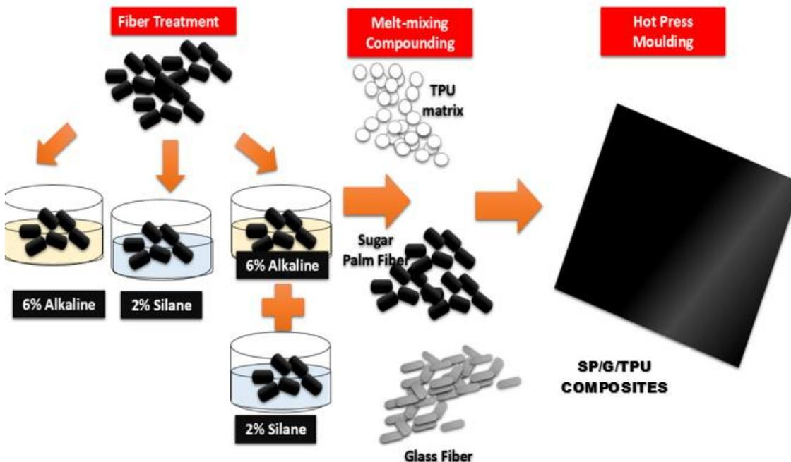
**Fig. 1.** Development of untreated and treated hybrid SPF/GF-reinforced TPU hybrid composites
