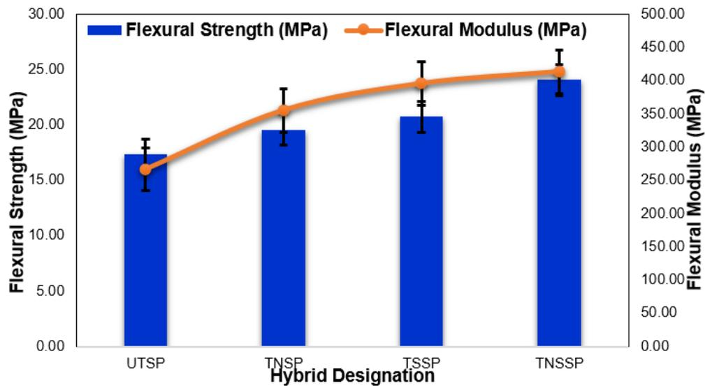
**Fig. 4.** Flexural properties of untreated and treated SPF/GF-reinforced TPU hybrid composites
