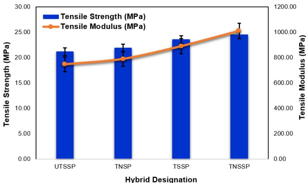
Fig. 2. Tensile properties of untreated and treated hybrid SP/G-reinforced TPU composites
