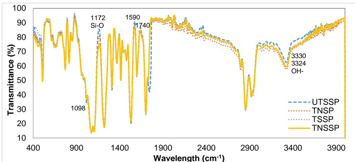
Fig. 6. FTIR spectra for UTSSP, TNSP, TSSP, and TNSSP
