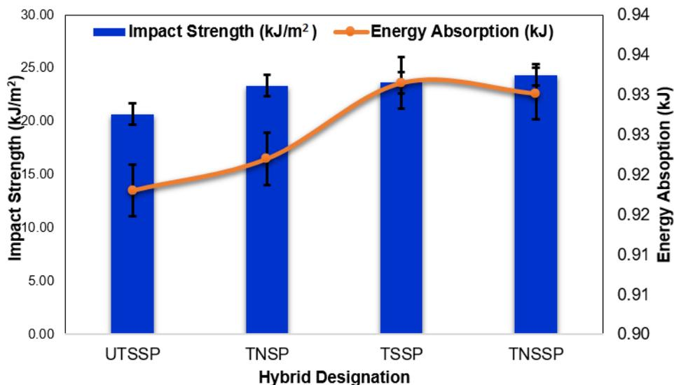
**Fig. 5.** Impact properties of untreated and treated hybrid SPF/GF-reinforced TPU composites
