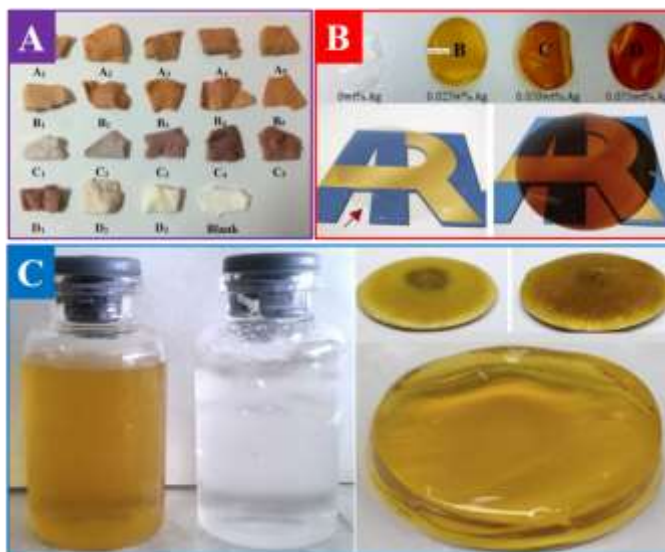
Fig. 7. AgNPs contained in various products: (A) paper (reprinted with permission from Xu et al. 2015), (B) NFC membranes (reprinted with permissions from Dong et al. 2013 and Ramaraju et al. 2015), and (C) NFC gels (reprinted with permissions from Dong et al. 2013 and Das et al. 2015)
