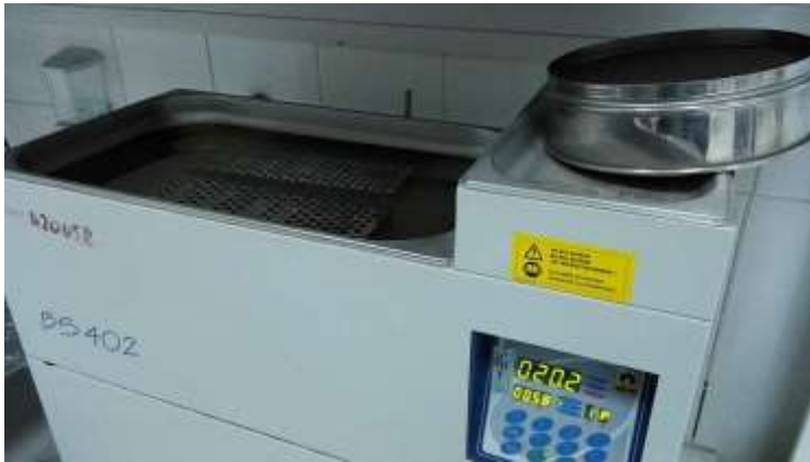
Fig. 3. Equipment used to determine the swelling in thickness after water immersion
