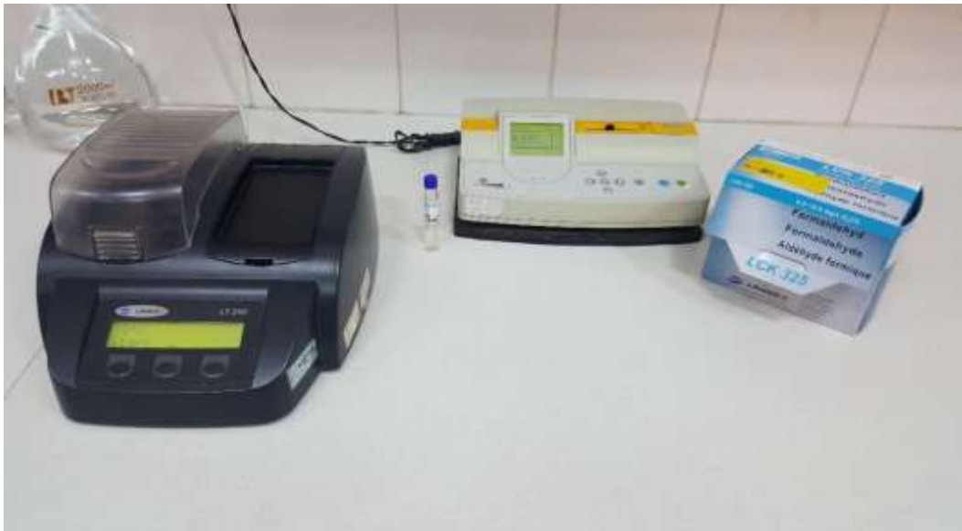
Fig. 2. Equipment to measure formaldehyde emission photometrically by the acetyl-acetone method
