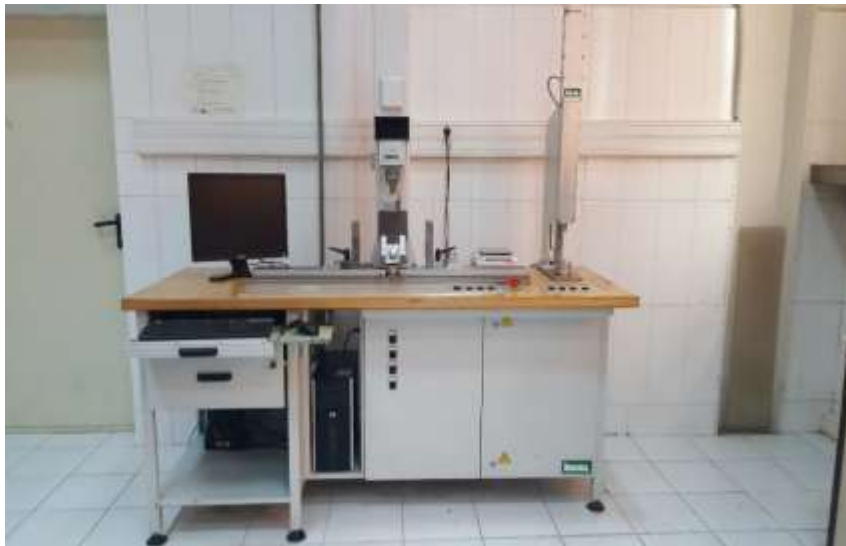
Fig. 5. Equipment used to determine the bending strength and modulus elasticity in bending
