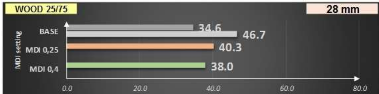
Fig. 8. Influence of board density and additive on the surface absorption, in mm
