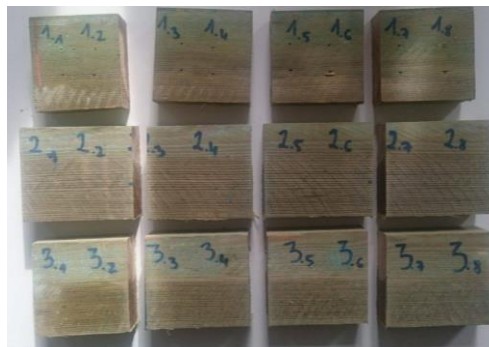
Fig. 4. The view of samples prepared for experiment: a) untreated, sawnwood, b) impregnated wood
