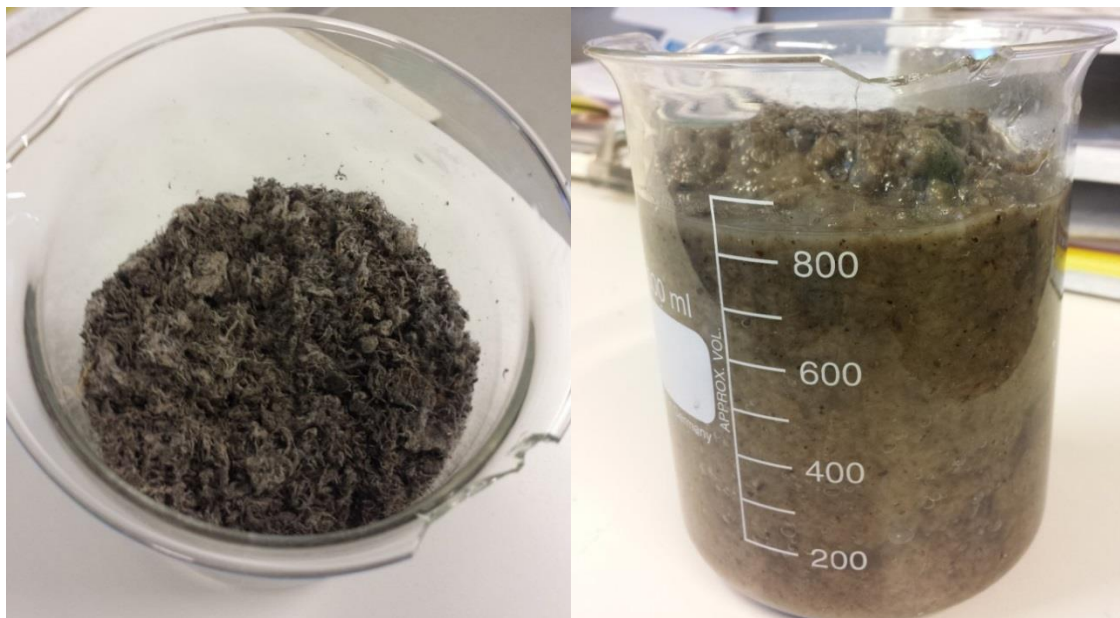
Fig. 2. Native and biotechnologically modified wood fiber sludge
