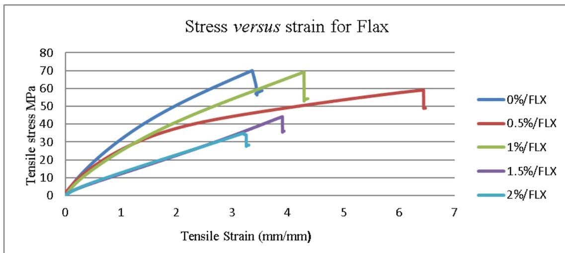
Fig. 4a. Stress-strain curves for flax with all five respective percentages of CNT
