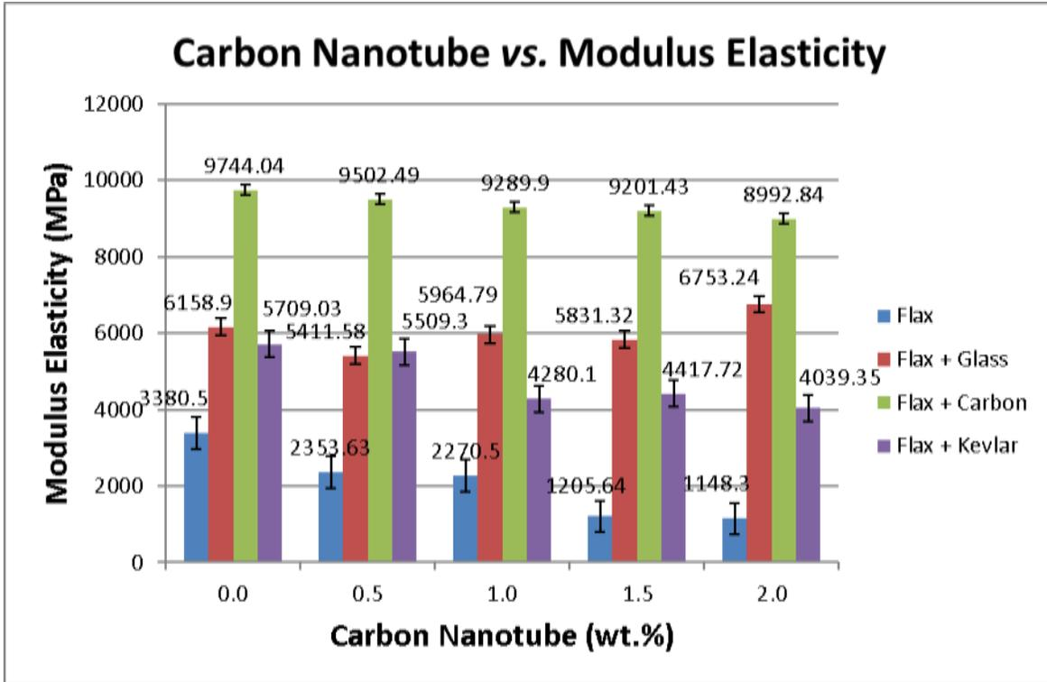
Fig. 4f. Tensile modulus of elasticity
