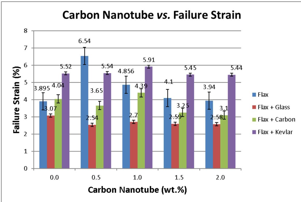
Fig. 4g. Failure strain
