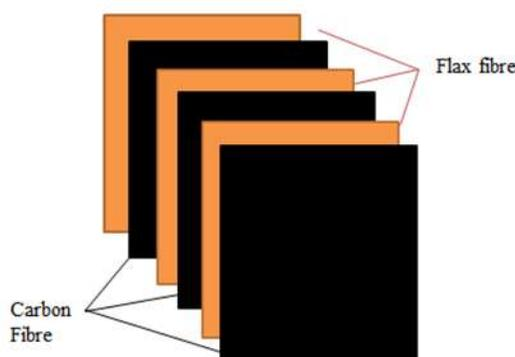
Fig. 2. Arrangement of fabricated hybrid biocomposite
