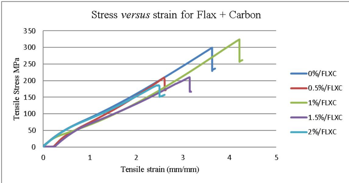
Fig. 4c. Stress-strain curves for flax + carbon hybrid with all respective percentages of CNT
