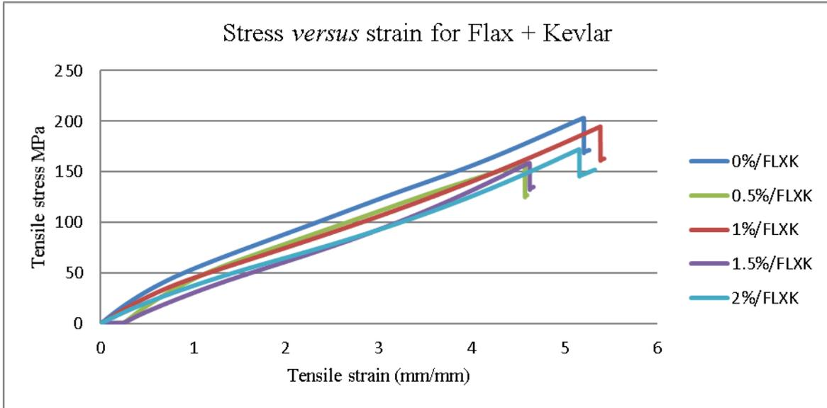
Fig. 4d. Stress-strain curves for flax + aramid hybrid with all five respective percentages of CNT
