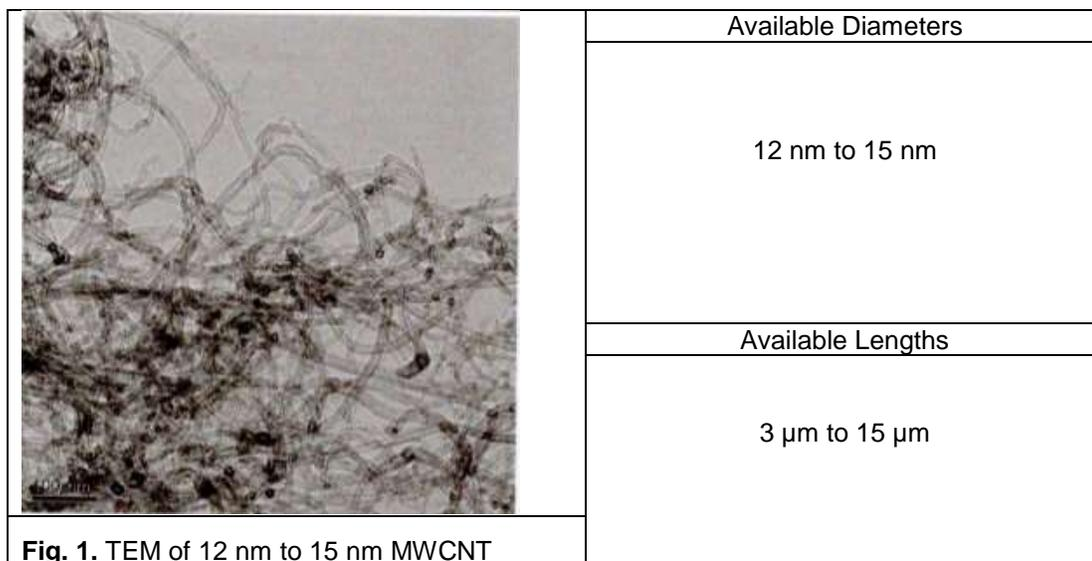
**Table 2.** Details of Multi-walled Carbon Nanotube
