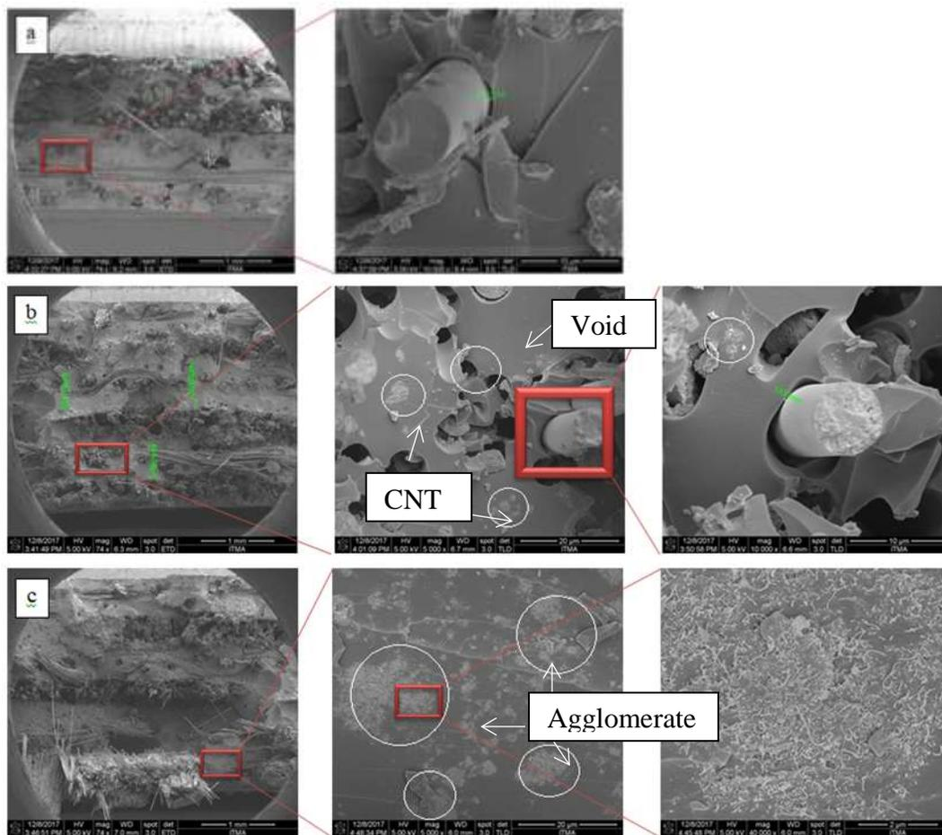
**Fig. 3.** FESEM images of the fracture area of (a) 0%/FLXC, (b) 1%/FLXC, and (c) 2%/FLXC
