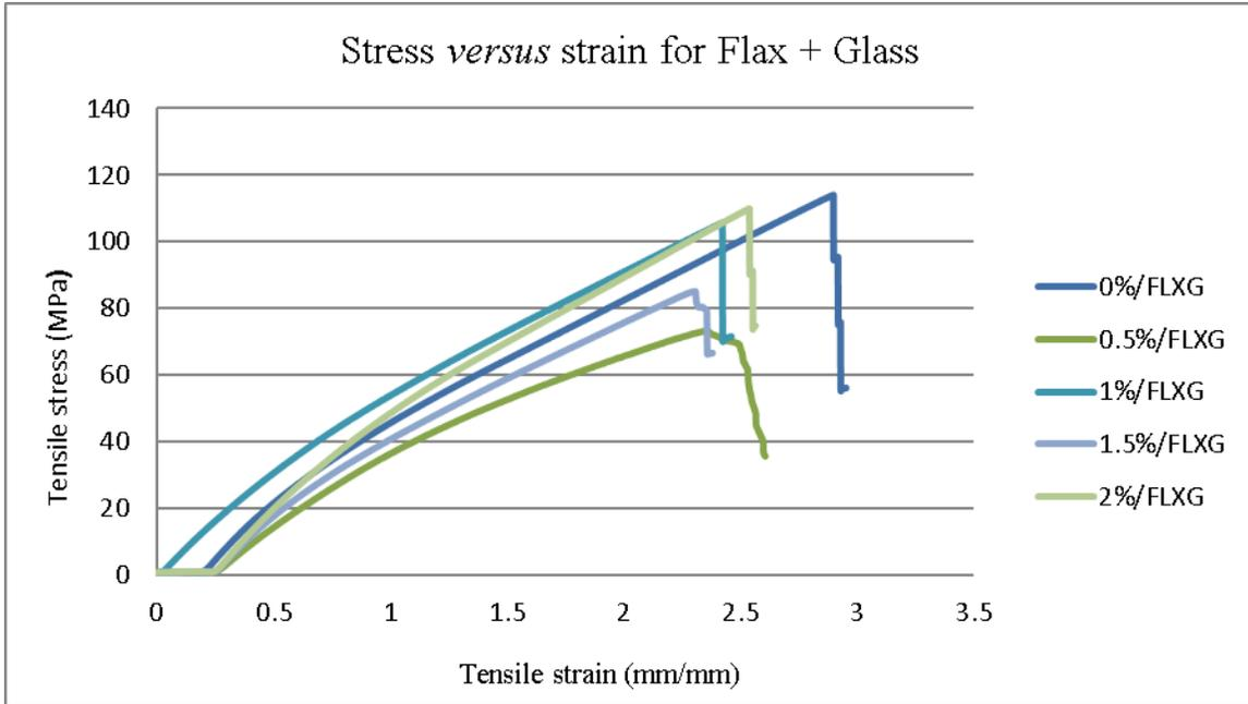
Fig. 4b. Stress-strain curves for flax + glass hybrid with all five respective percentages of CNT
