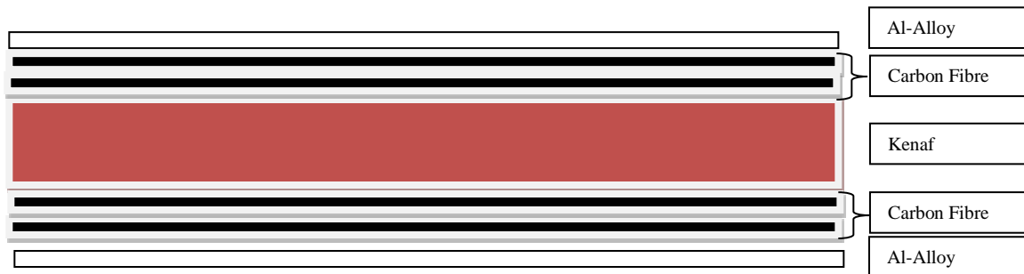
Fig. 1. FML of the aluminium alloy with carbon and kenaf fibres
