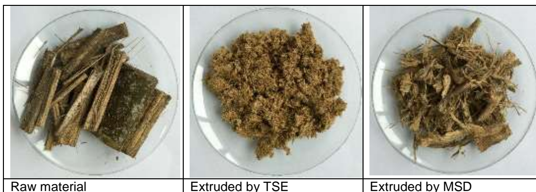
Fig. 4. Outward appearance of raw material and extruded materials
