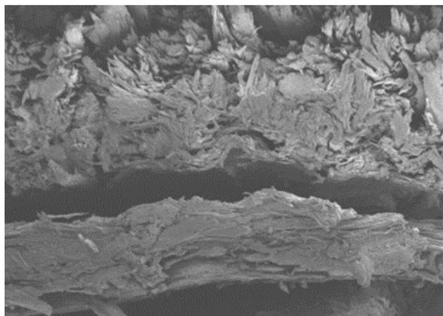
(b) Cross-section of the damaged laminated veneer lumber ( $\times 70$ , 500  $\mu\text{m}$ )
