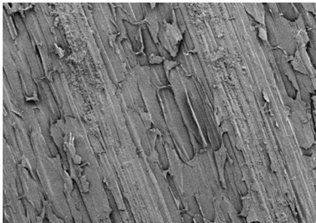
(a) Torn and adhesive layers ( $\times 100$ , 500  $\mu\text{m}$ )
