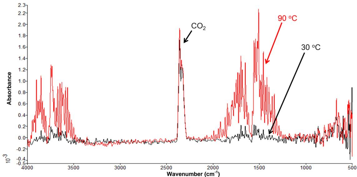
Fig. 2. The FT-IR spectra of corn stalk rind after gluing at 30 °C and 90 °C
