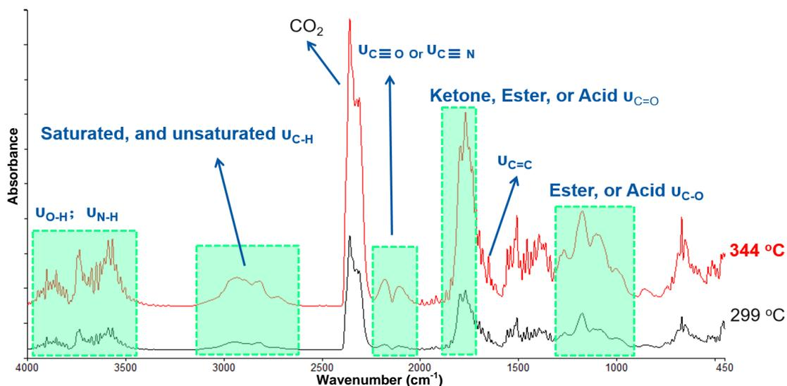
Fig. 3. The FT-IR spectra of corn stalk rind after gluing at 299 °C and 344 °C
