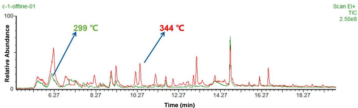
Fig. 4. GC-MS chromatogram of corn stalk rind after gluing at 299 °C and 344 °C
