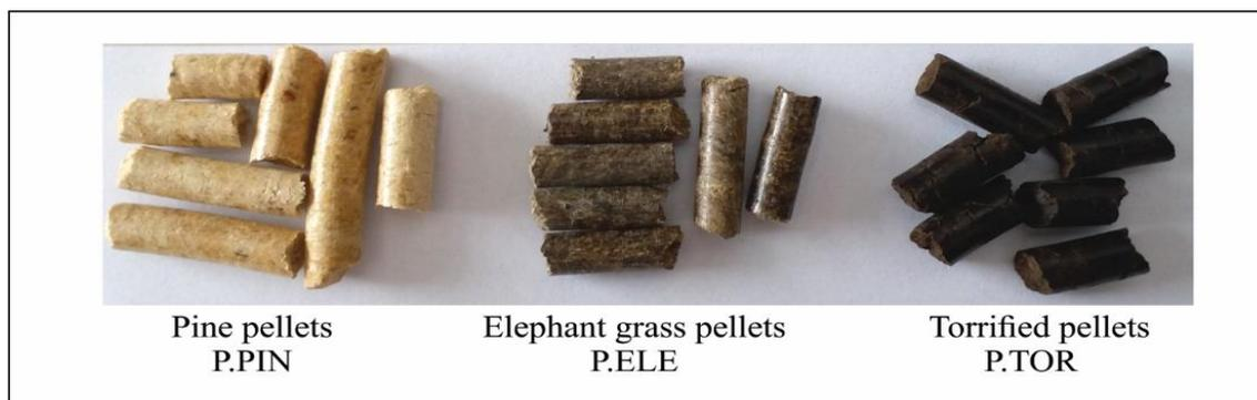
**Fig. 2.** Samples of plant biomass pellets used for the tests
