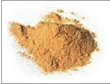
Fig. 1. Beech wood dust sample after grinding with sandpaper
