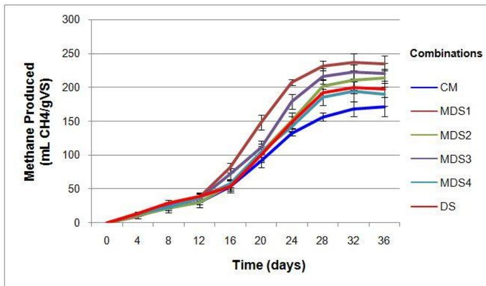
Fig. 5. Methane production from co-digestion of DSL and CM
