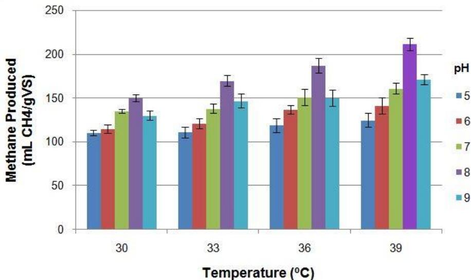
Fig. 2. Results of methane production from MDL during pH and temperature optimization
