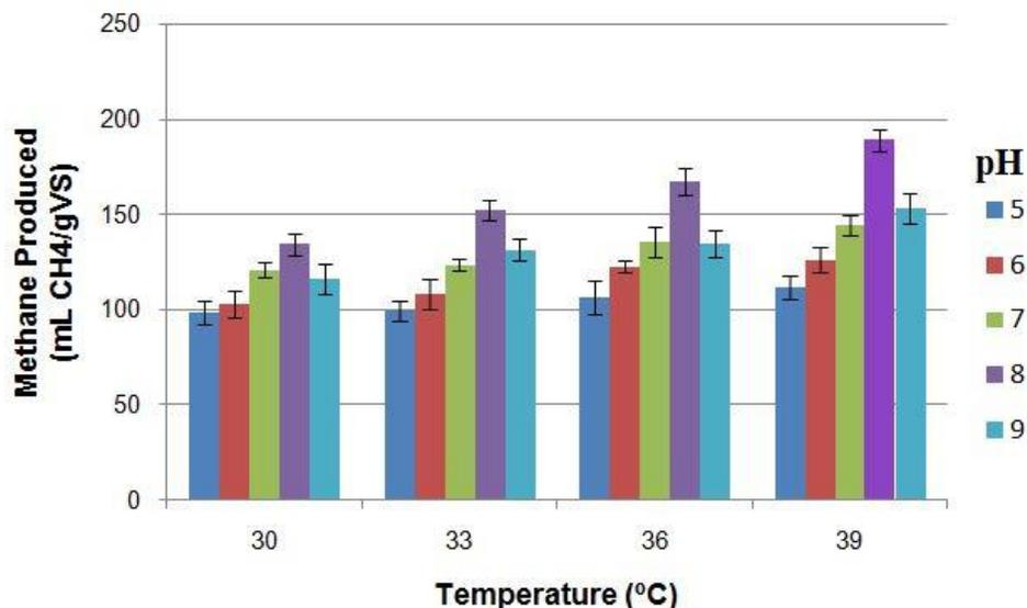
**Fig. 3.** Results of methane production from DS during pH and temperature optimization
