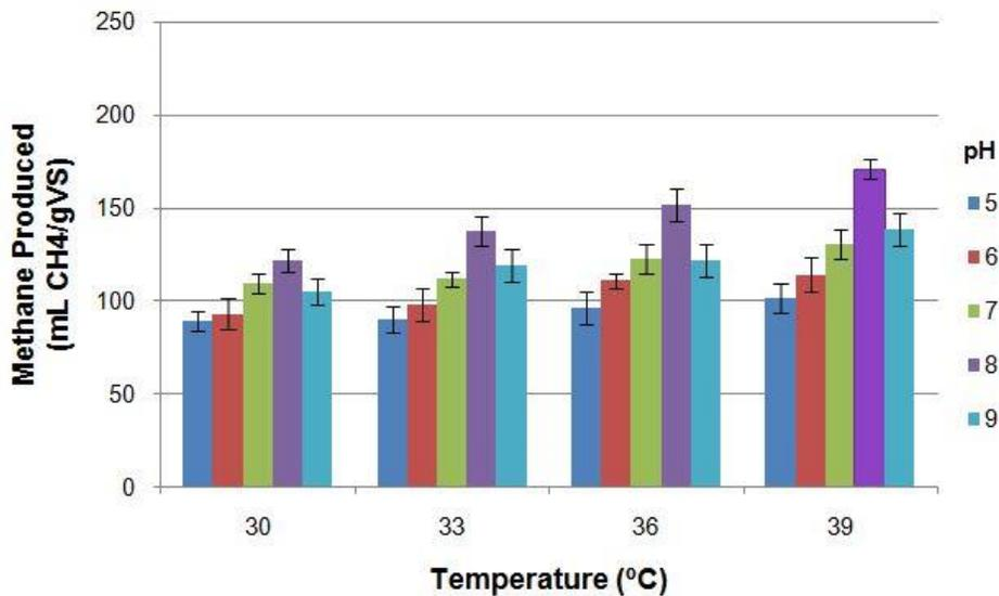
Fig. 1. Results of methane production from CM during pH and temperature optimization
