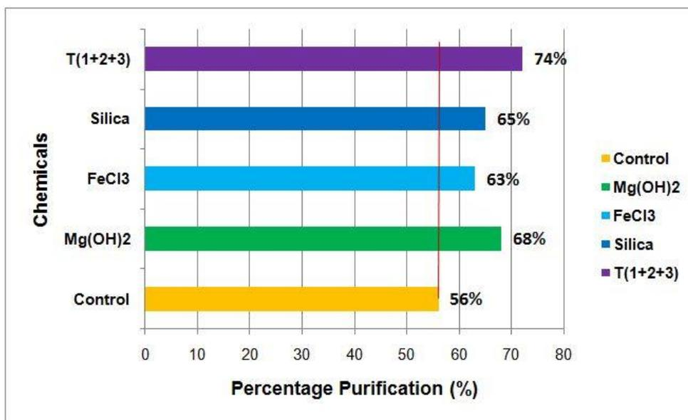
Fig. 6. Chemical treatments for biogas purification
