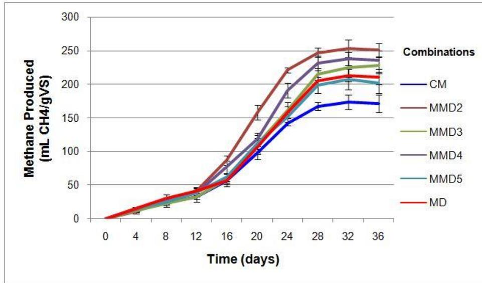
Fig. 4. Methane production from co-digestion of MDL and CM
