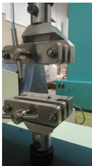
Fig. 3. Testing of tensile characteristics of abaca fibres
