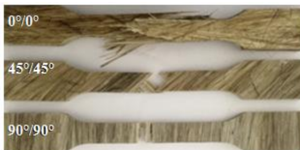
Fig. 10. Different types of failures of specimens
