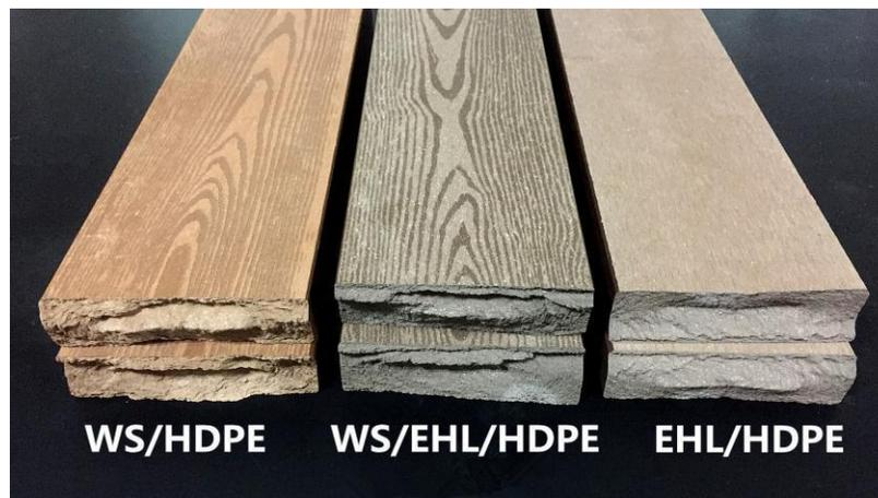
**Fig. 1.** The fractured end surfaces of different composite pilot-products
