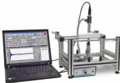
Fig. 2. PC-based technology Sonelastic® equipment. Source: Sonelastic® (2011).
