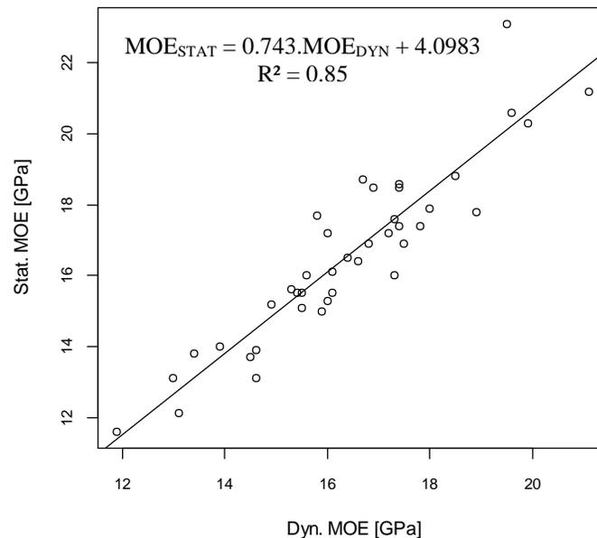
**Fig. 5.** Linear regression of the dynamic and static modulus of elasticity
