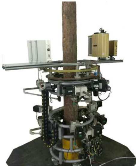
Fig. 1. A nondestructive testing system for living trees
