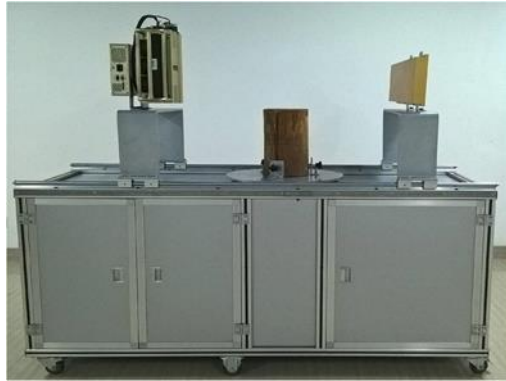
Fig. 3. A nondestructive testing system for wood
