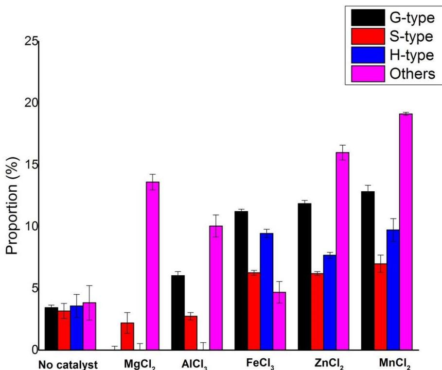
**Fig. 4.** The proportion of different types of phenolic monomer in all monomers of the lignin depolymerization products
