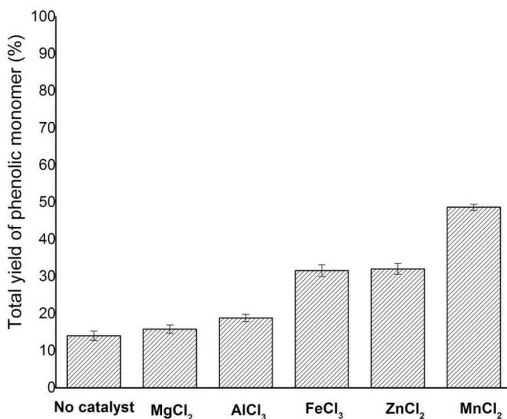
**Fig. 3.** The percentages of total monomer content of lignin depolymerization generated by different catalysts
