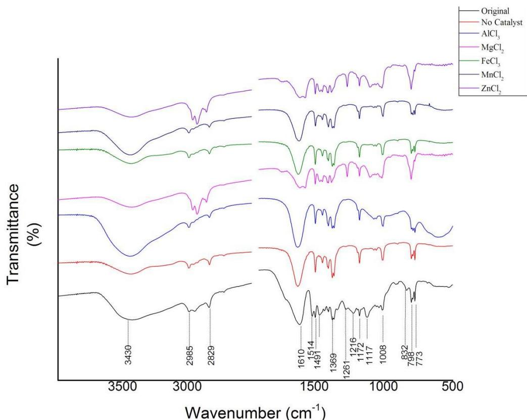
**Fig. 5.** FT-IR spectra of the lignin before and after depolymerization with various metal chloride catalysts
