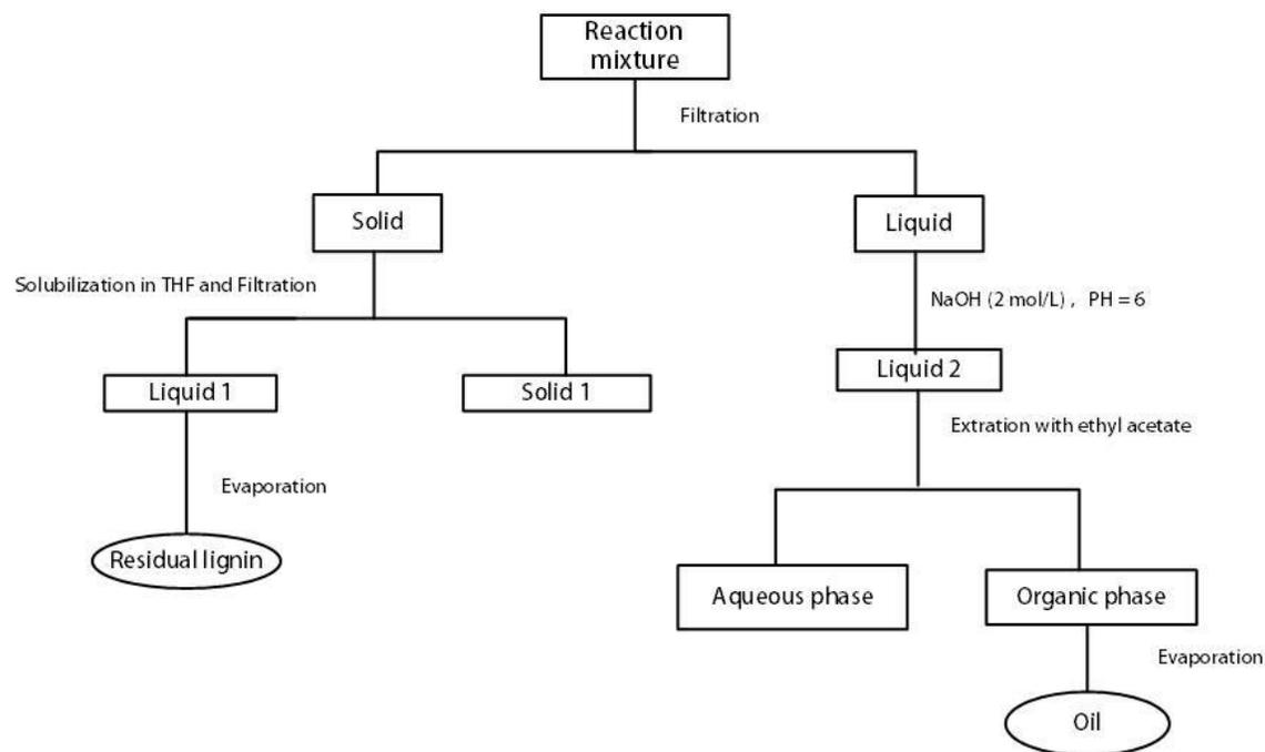
**Fig. 1.** Schematic process of lignin depolymerization and separation of the reaction products
