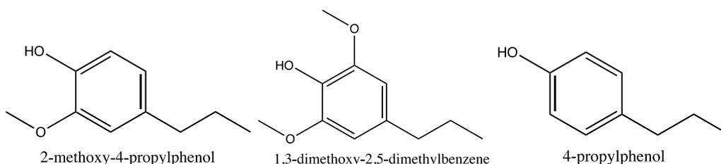
**Fig. 2.** Three basic phenyl propane structure units of lignin
