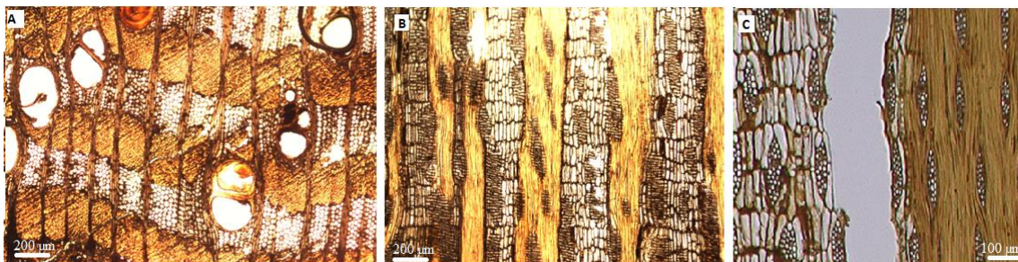
Fig. 3. Micrographs of M. stuhlmannii : (A) Transverse section view; (B) Radial longitudinal view; and (C) Tangential longitudinal view
