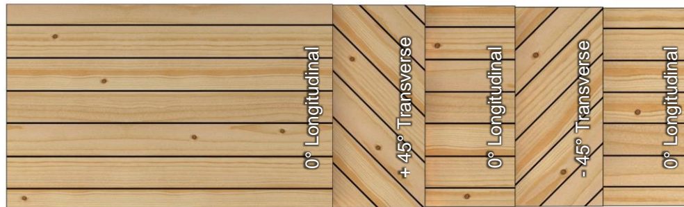
Fig. 4. Schematic of the configuration of a five-layered CLT panel with 0° longitudinal and \pm 45^\circ transverse layers
