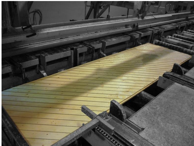
Fig. 5. Industrial modified production of CLT ± 45° panels
