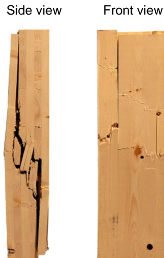
Fig. 7. Uniaxial compression test sample: side and front views of crushing and axial splitting failure in the same CLT 90^\circ sample
