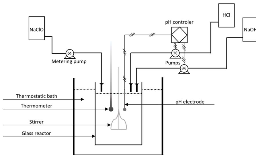
**Fig. 1.** aTEMPO mediated oxidation experimental setup
