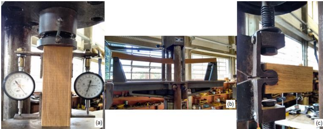
Fig. 1. Cupiúba specimen: (a) compression parallel to grain; (b) static bending; (c) cleavage strength
