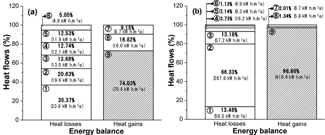
**Fig. 2.** Annual heat losses and heat gains of (a) WFH, (b) Hanok by component (① windows; ② Exterior wall; ③ Roof; ④ Floor slab; ⑤ Exterior door; ⑥ Ventilation; ⑦ Internal heat gain; ⑧ Solar gain; ⑨ Heating demand)
