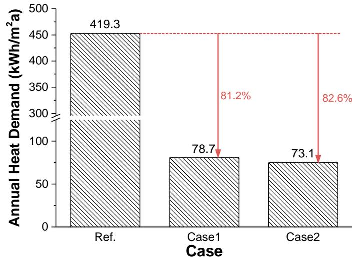
Fig. 4. Heating Energy Reduction of Hanok by Case
