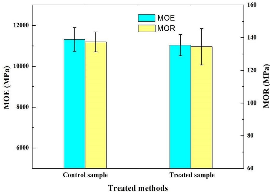
Fig. 13. Comparative values of mechanical properties of bamboo from control and treated state
