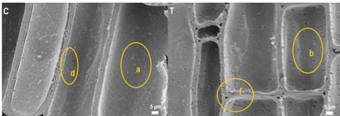
**Fig. 9.** Single comparison of the parenchyma cells for control (C) and treated (T) bamboo
