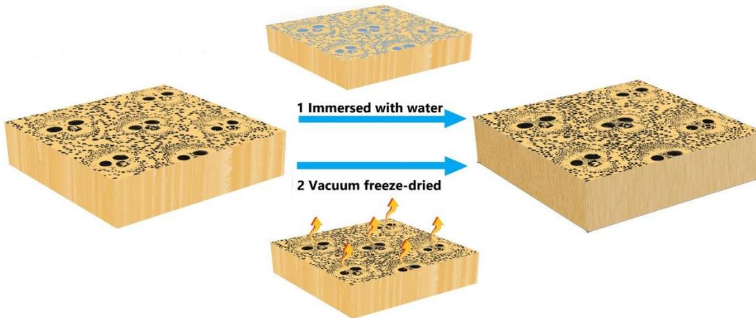
Fig. 2. Preparation of porous bamboo by vacuum freeze-drying
