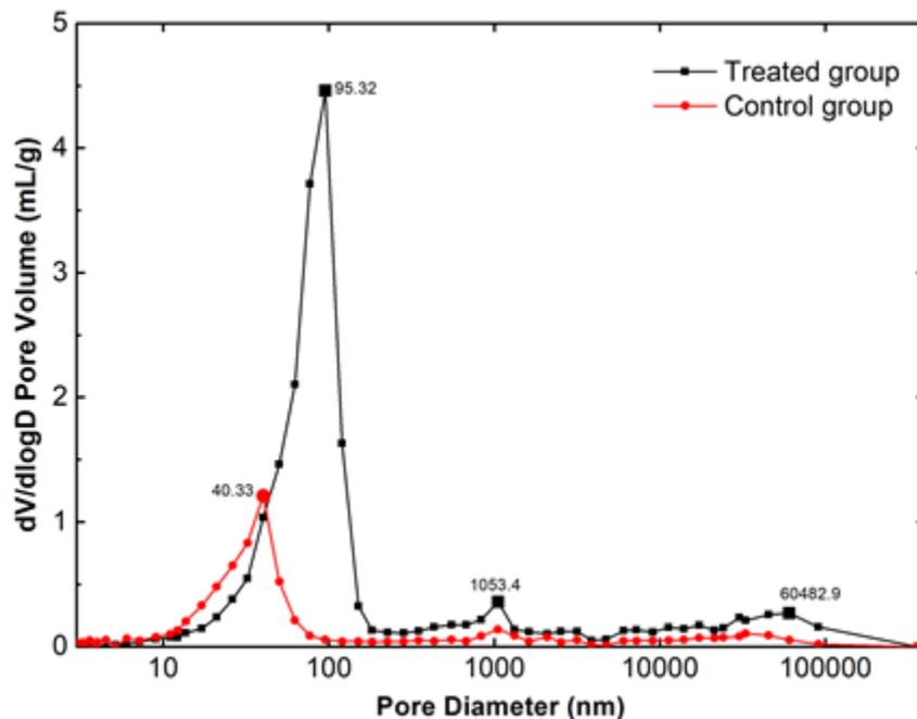
Fig. 11. Log-differential intrusion as a function of the pore diameter of bamboo
