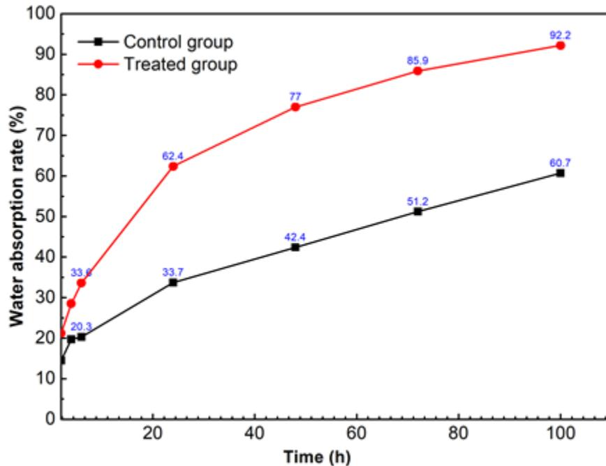
Fig. 6. Water absorption rate of bamboo samples for C (control) and T (treated) bamboo
