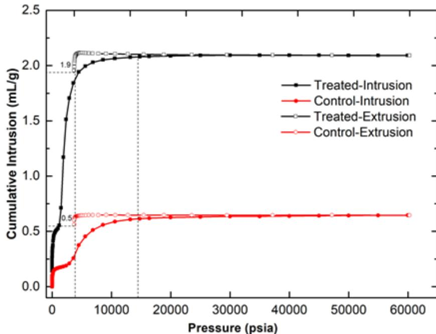
Fig. 12. Cumulative pore volume as a function of the pressure of one intrusion-extrusion cycle
