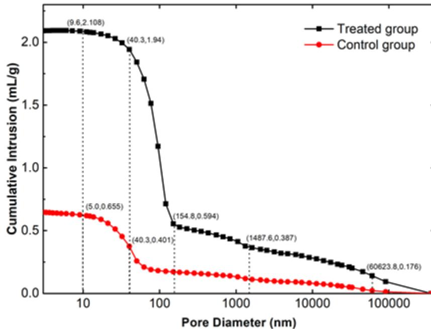
Fig. 10. Cumulative pore volume as a function of the pore diameter of bamboo
