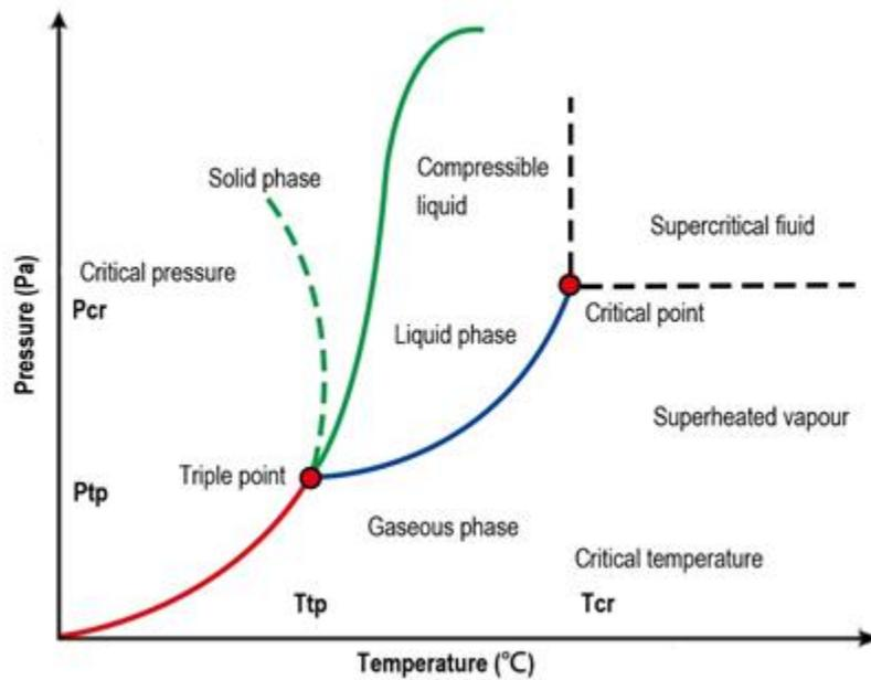
Fig. 1. Three-phase diagram of water (Xu *et al.* 1994; Han 2007)
